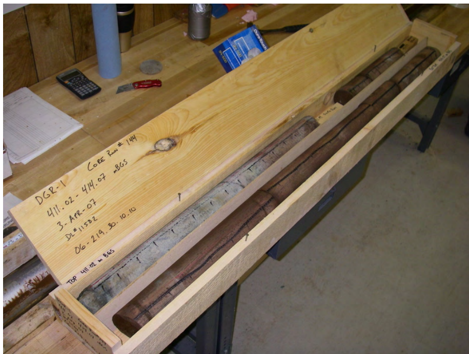
Figure 3.24 Top of Cabot Head Formation shale, 411.02 to 414.07 mBGS in DGR-1
