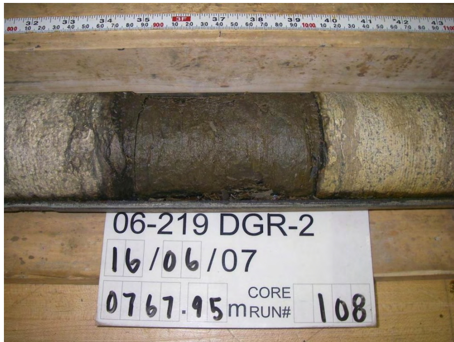
Figure 3.38 Volcanic ash bed, Coboconk Formation, 768.6 m BGS, DGR-2
