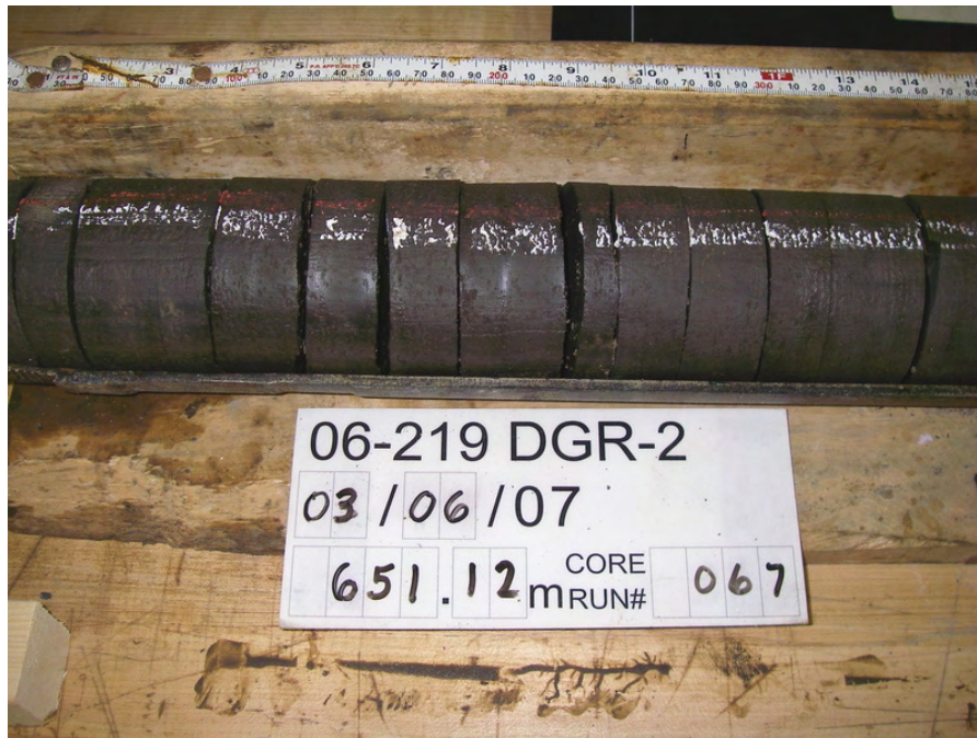
Figure 3.33 Core diskings of Lower Member, Blue Mountain Formation shale, 652 mBGS, DGR-2
