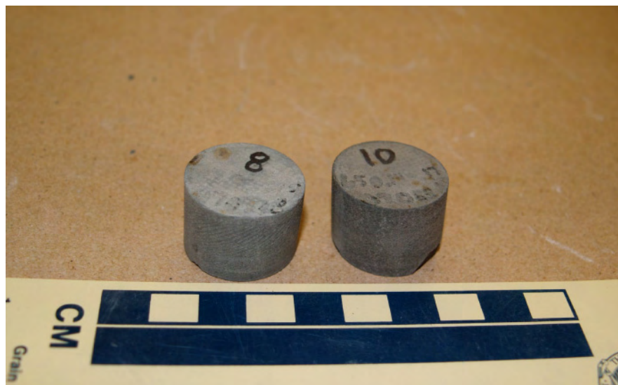
Figure 4.17 Core plugs from DGR2-613.93 (left) and DGR2-650.12 (right) in Blue Mountain Formation had measured vertical permeabilities of 6\text{E-}16 and 9\text{E-}16 \text{ m}^2 . Hydraulic testing of these intervals yielded in-situ values of \sim 1\text{E-}21 \text{ m}^2 .
