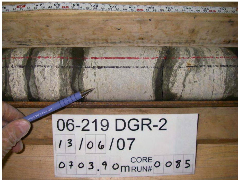
Figure 3.37 Core sample of Lower Member of Sherman Fall argillaceous limestone, 703.90 mBGS, DGR-2
