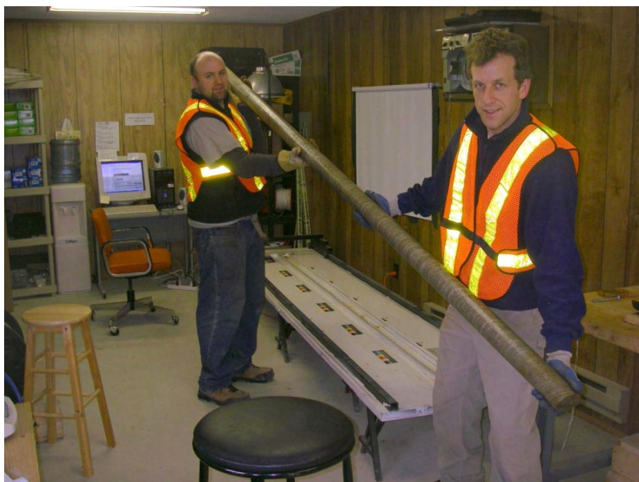
Figure 3.21 Intact 3.0 m length core of the Salina A0 Unit Dolostone at 371-374 mBGS in DGR-1
