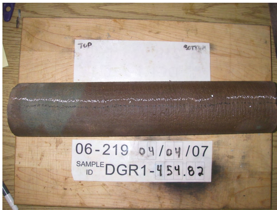
Figure 3.27 Core sample of green and red shale, upper Queenston Formation, 454.82 mBGS, DGR-1
