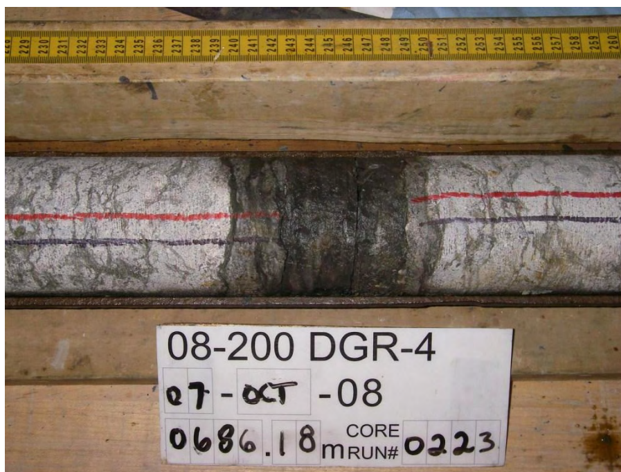
Figure 3.54 Fractured fissile shale layer at a depth of 688.6 mBGS in the bottom of the Cobourg Formation, DGR-4
