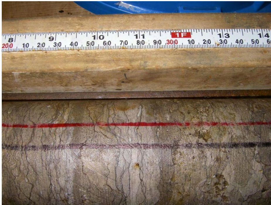
Figure 3.39 Trace of hydrocarbon weeping from stylolites, Gull River Formation, 817.0 mBGS in DGR-2
