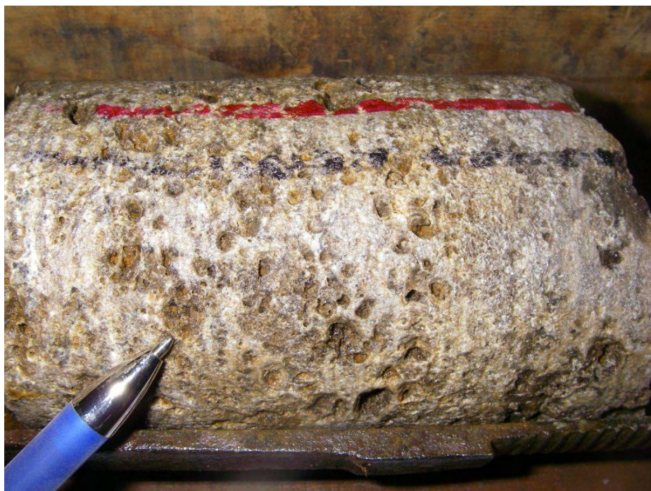
Figure 3.20 Open vuggy porosity of Upper A1 Unit Carbonate Unit at 326.2 mBGS in DGR-4
