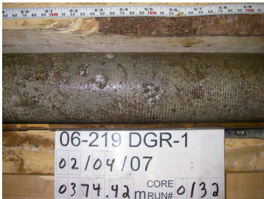
Figure 3.23 Core photograph of Guelph Formation porous dolostone at 376 mBGS in DGR-1
