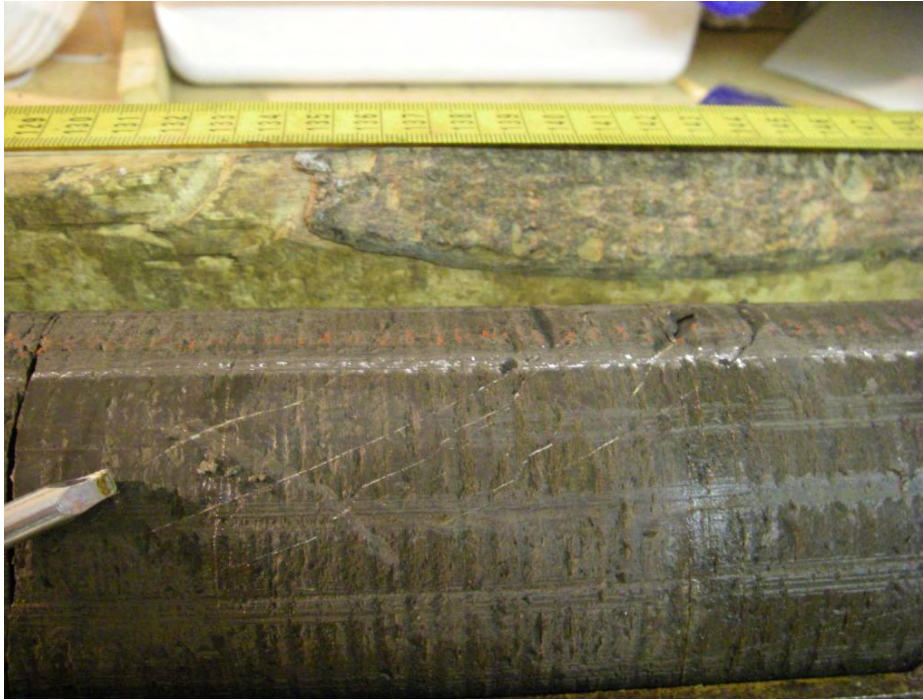
Figure 4.91 Closely-spaced, inclined, calcite-infilled fractures at 638.5 mBGS in Blue Mountain Formation, DGR-3. Note pitting or minor core breakage at the low point on the elliptical fracture trace.
