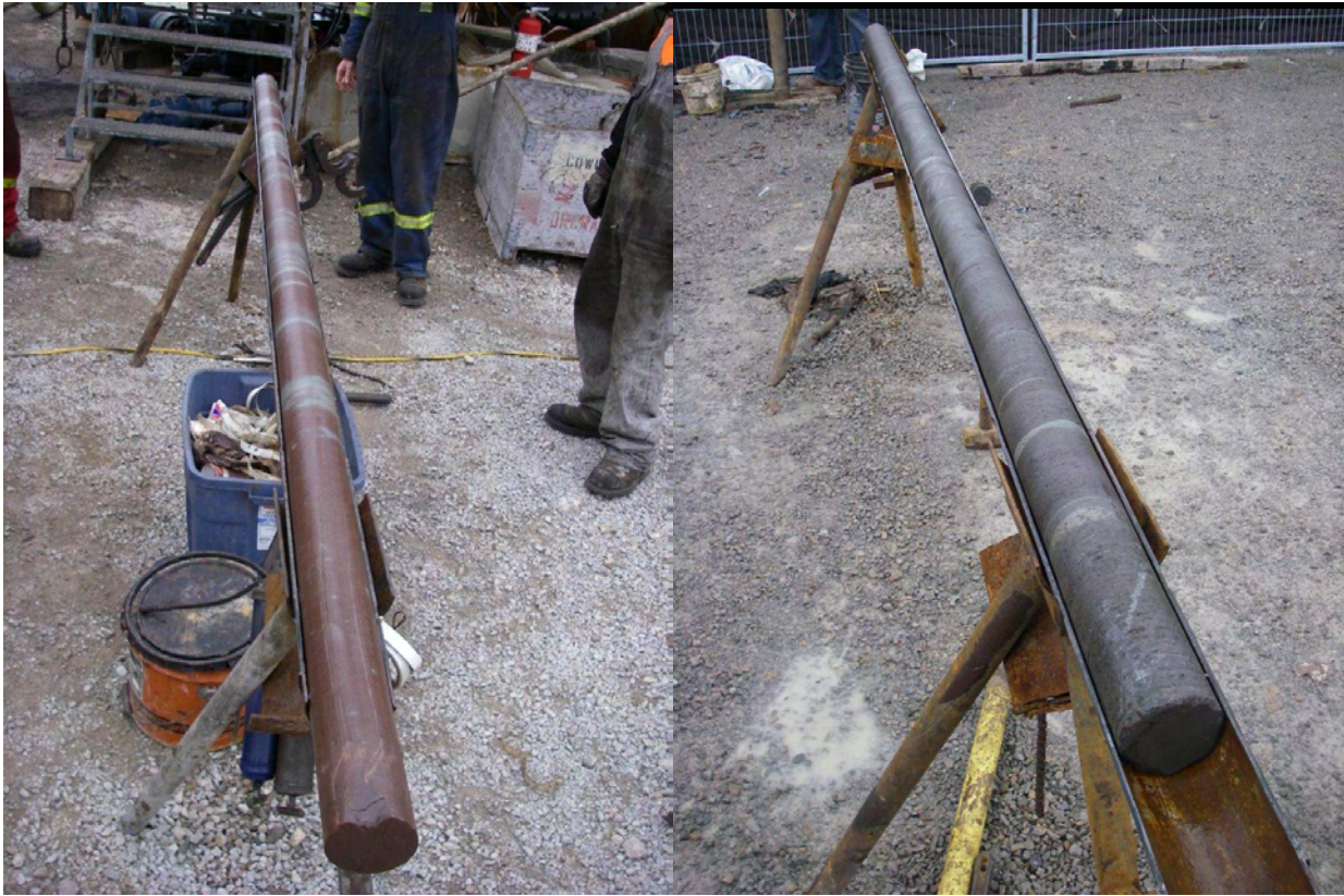
Figure 3.30 Intact core runs: left - Queenston Formation, 475.73-478.78 mBGS in DGR-3, right - Blue Mountain Formation, 619.08-622.13 mBGS in DGR-4
