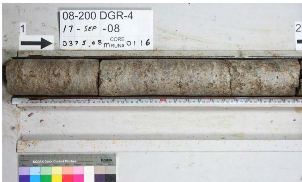
Figure 4.83 Permeable vuggy core in Guelph Formation dolostone, 375 mBGS, DGR-4
