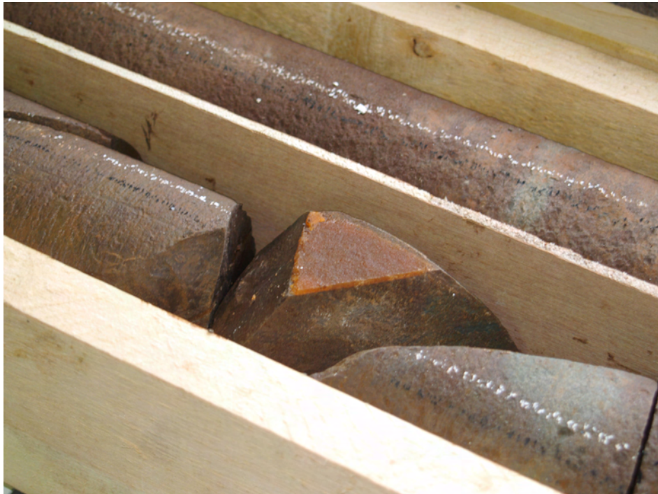
Figure 3.43 Orange halite and calcite fracture infill in the Queenston Formation shale at 456.01 mBGS in DGR-1
