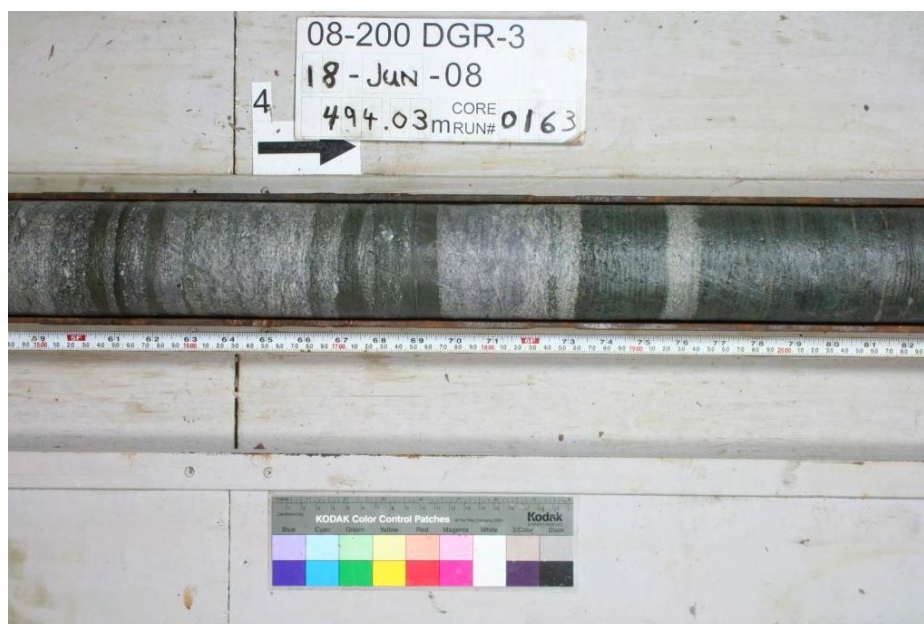
Figure 3.29 Interbedded green shale and grey fossiliferous limestone, middle Queenston Formation at 496 mBGS in DGR-3
