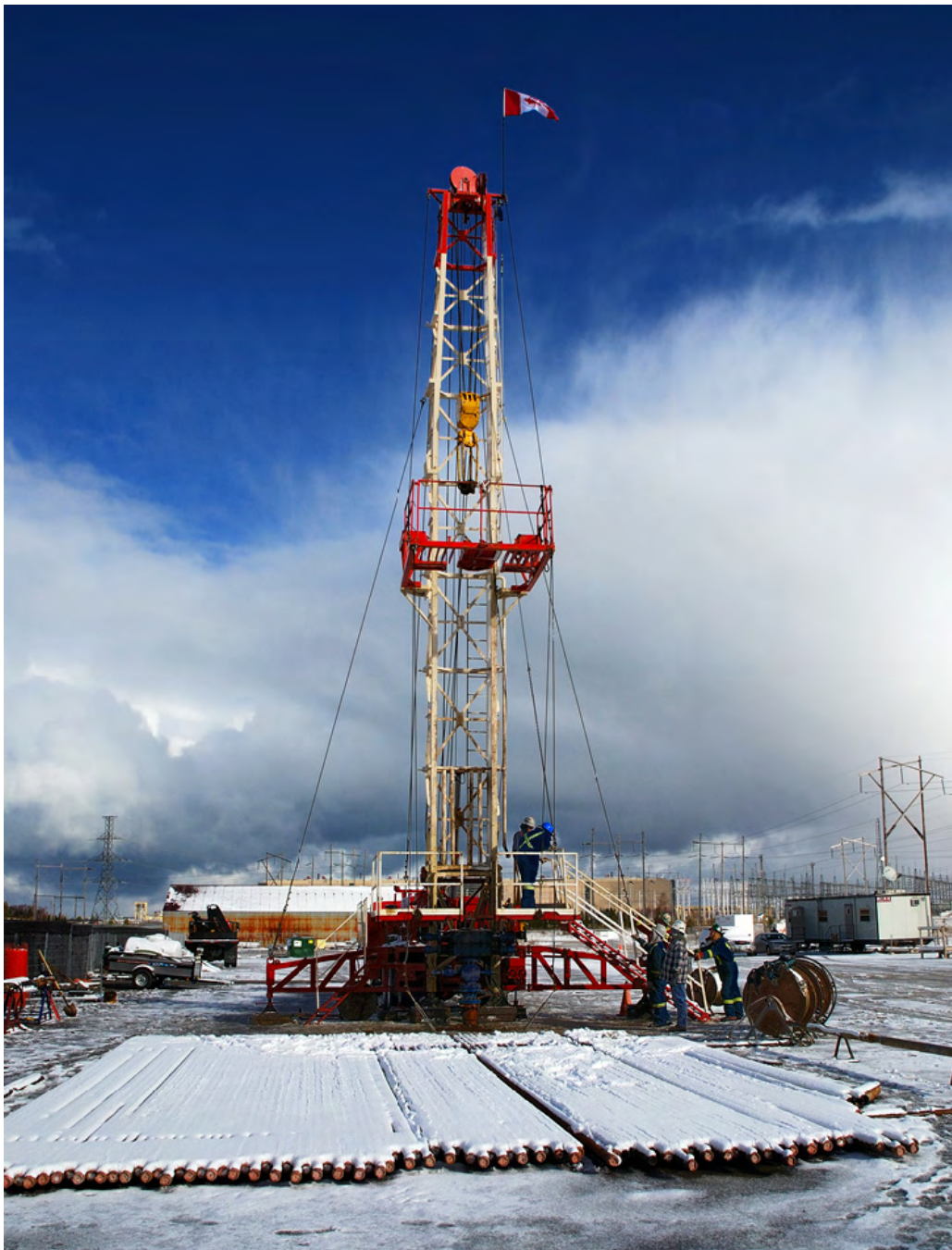
Figure 4.74 Straddle-packer hydraulic testing at DGR-4 using workover rig and drill tubing
