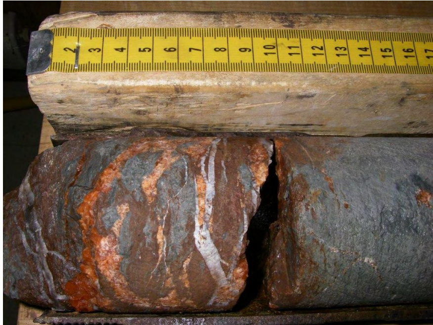
Figure 3.17 Orange anhydrite veins cut by white gypsum veins in Salina F Unit dolomitic shale, 222.6 mBGS in DGR-3.
