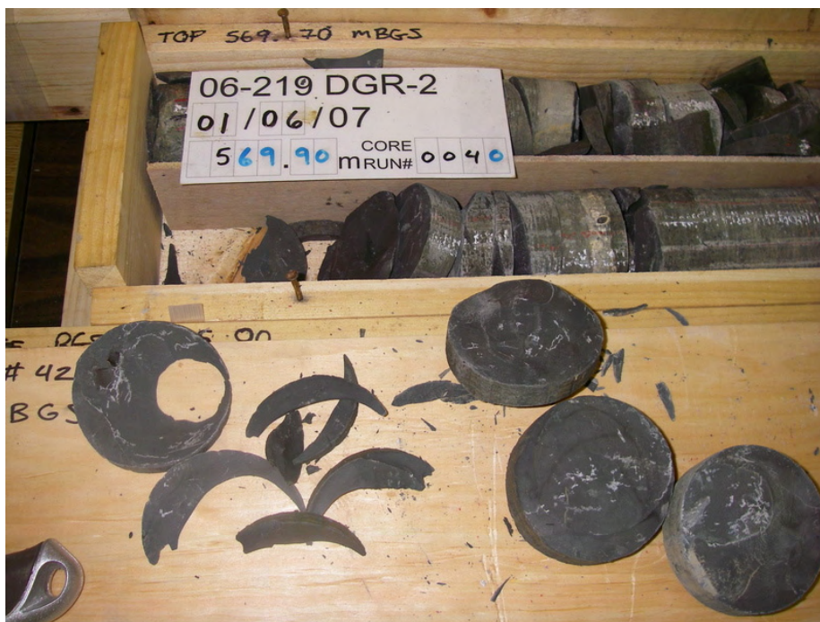
Figure 3.32 Core diking in upper Georgian Bay Formation shale, 569.90 mBGS, DGR-2
