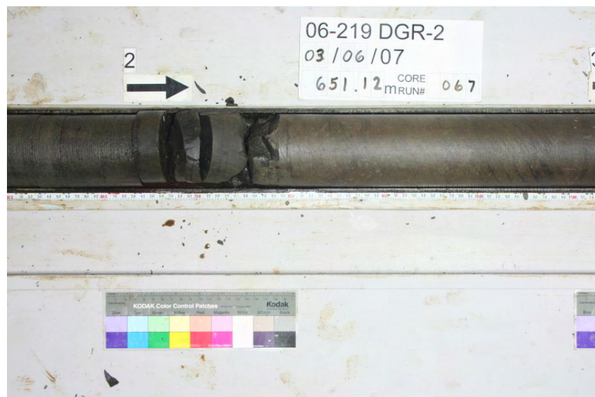
Figure 3.34 Contact between dark grey Blue Mountain Formation and brownish-grey Collingwood Member of the Cobourg Formation, 651.6 mBGS in DGR-2
