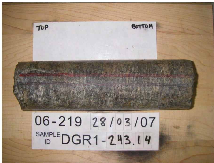
Figure 3.18 Core sample of Salina D Unit anhydritic dolostone from 243.14 mBGS in DGR-1
