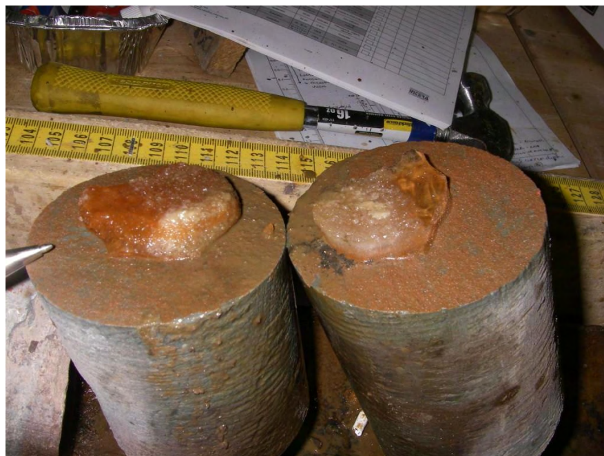
Figure 3.26 Halite-infilled horizontal fracture at 458.6 m BGS in upper Queenston Formation in DGR-3
