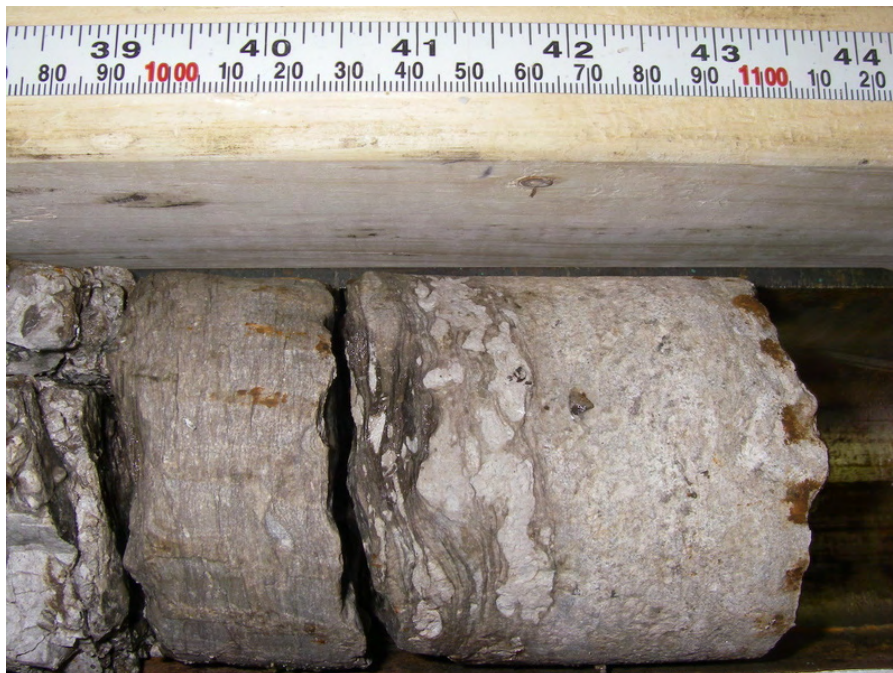
Figure 3.16 Core sample of Bois Blanc Formation cherty dolostone with bituminous laminations, 102.3 mBGS, DGR-1
