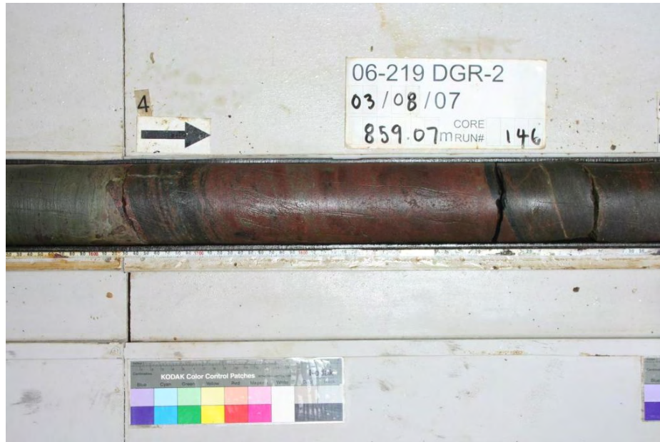
Figure 3.47 Contact between Cambrian Formation and PreCambrian basement at 860.70 mBGS in DGR-2, NB contact is at start of arrow
