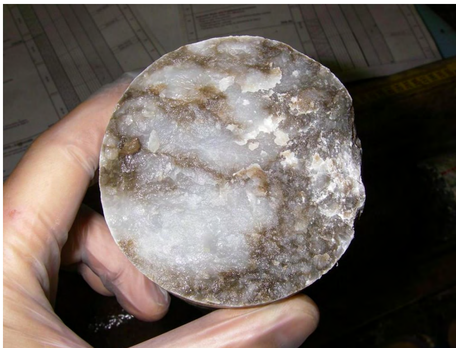
Figure 3.19 Dolomitic anhydrite of Salina A2 Unit Evaporite, 322.75 mBGS in DGR-4
