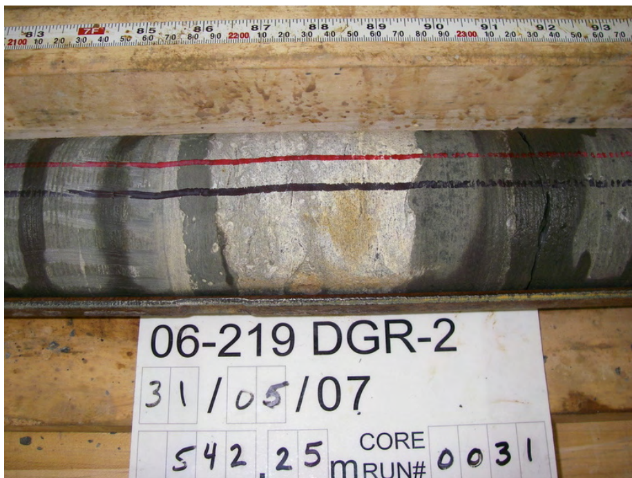
Figure 3.31 Core sample of upper Georgian Bay Formation interbedded shale and limestone, 542.25 mBGS, DGR-2
