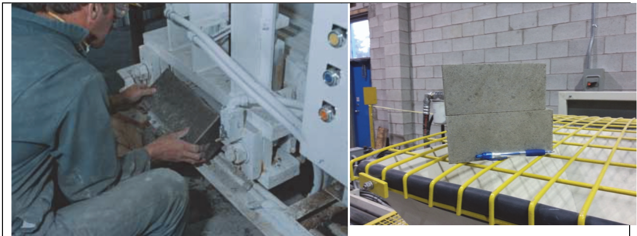
Figure 17: Portable uniaxial brick maker and trimmed HCB brick
