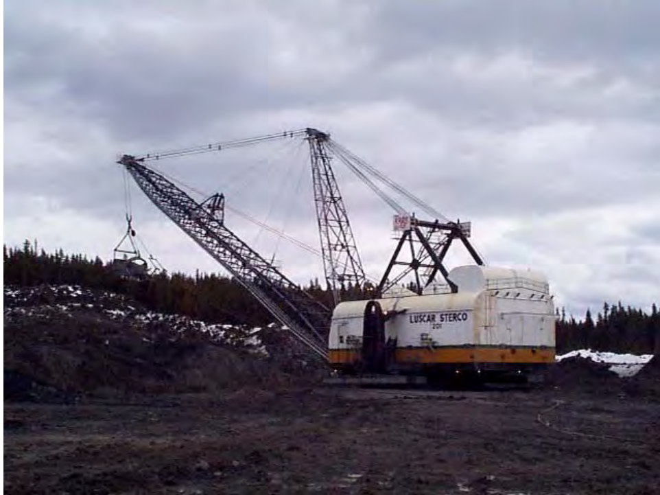
Figure 2 Dragline used to remove the overburden to expose the coal seam
