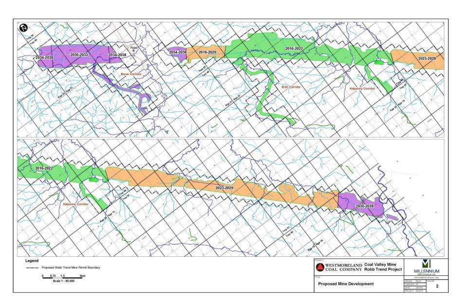
Development of the Robb Trend Mine is proposed to begin in the central portion of the mining area and progress to the outer portions.
