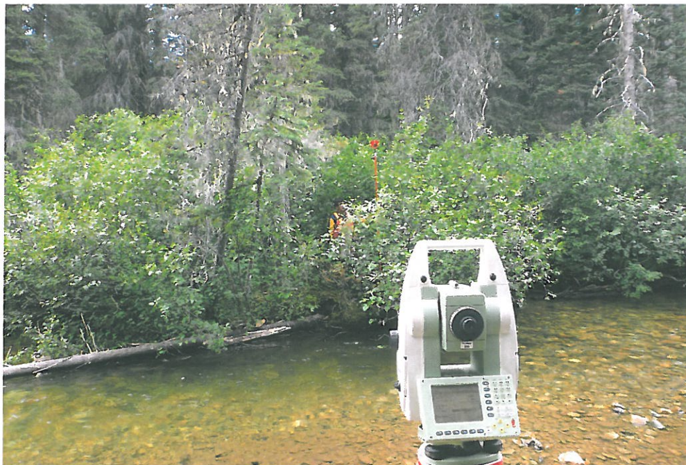
(Figure 4 –Leica TCR 1203 - Measuring to the target in thick vegetation)
