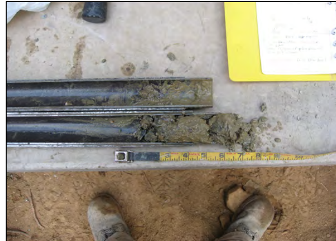
PHOTO 14 GT12-08 SPT #11 - 18.29m - 18.47m
