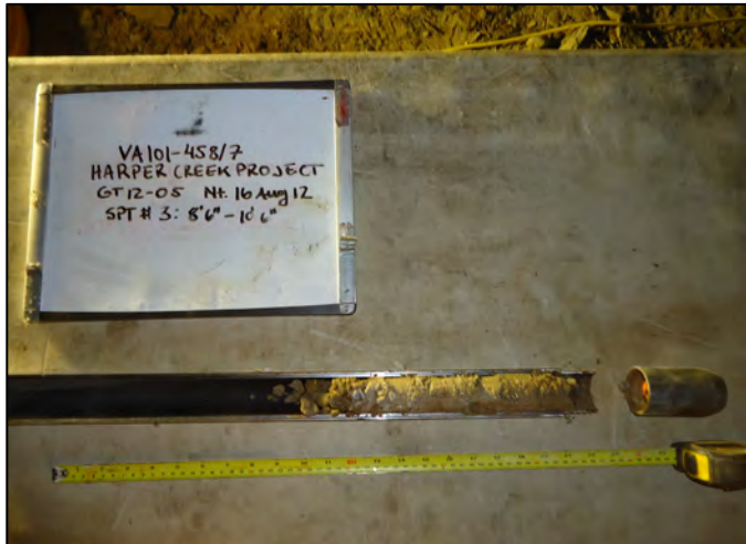
PHOTO 13 GT12-05 SPT#3 - 2.62m - 3.20m
