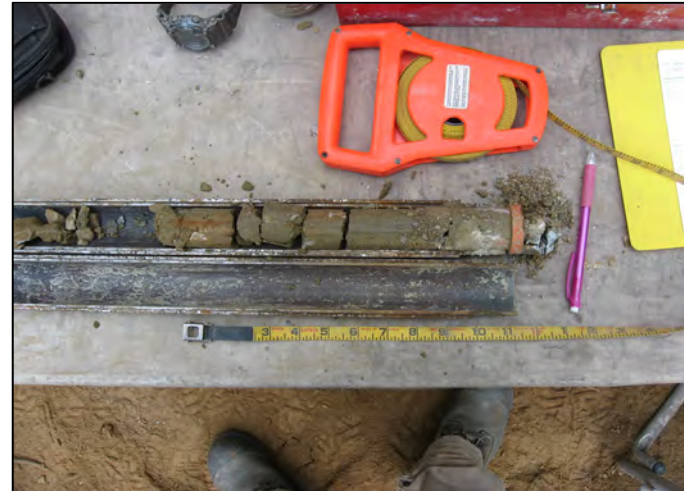
PHOTO 6 GT12-08 SPT #2 - 3.05m - 3.38m
