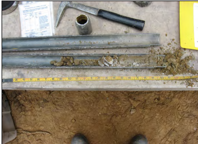
PHOTO 5 GT12-08 SPT #1 - 1.52m - 2.13m
