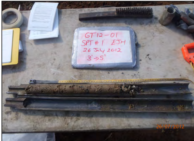
PHOTO 9 GT12-01 SPT#1 - 0.91m - 1.52m
