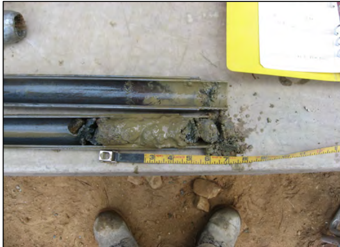
PHOTO 13 GT12-08 SPT #10 - 15.24m - 15.64m
