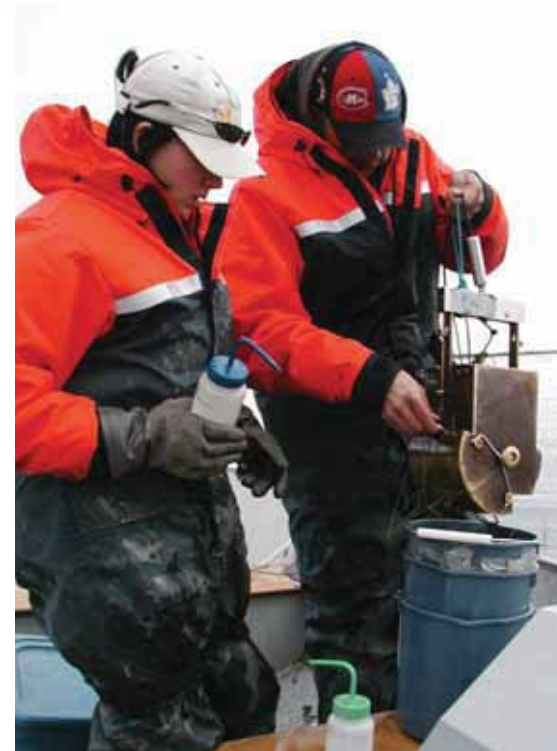
Collecting a benthic invertebrate sample with an Ekman dredge.
