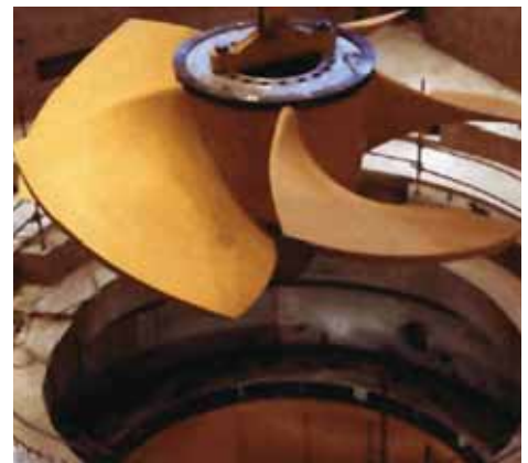
Keeyask turbines are designed to minimize fish injury and mortality.
