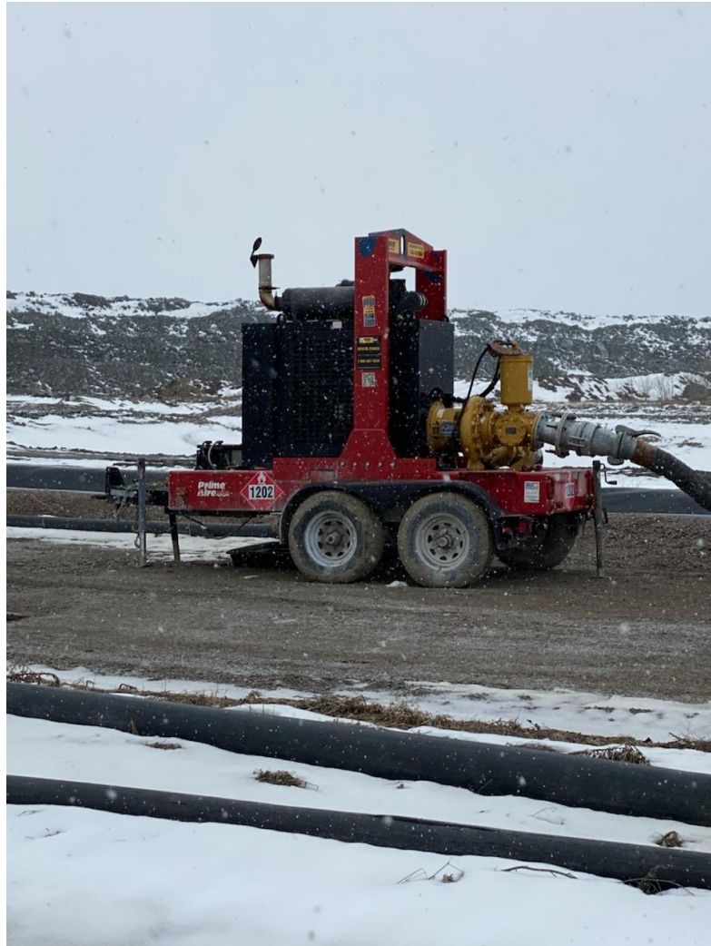
Figure 6 High-Volume pump installed to discharge water straight into tailings line and into the TMA.
