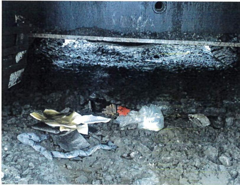
Photo 2. Spill cleanup pads, coils and trays used to contain and clean up hydraulic fluid spill.
