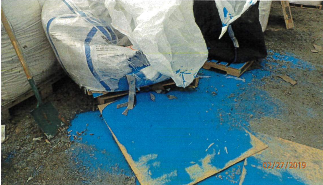
Figure 2. Copper sulphate tote bag with tear and spillage onto cold storage tent floor.
