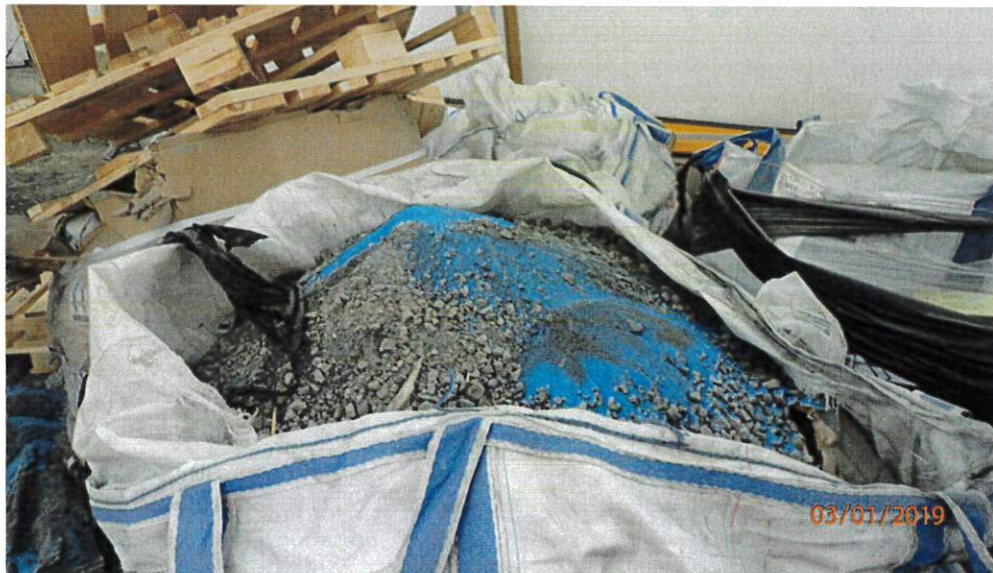
Figure 3. Spillage bag containing materials removed from the cold storage tent floor. Bag contains mixture of granular copper sulphate, gravel, clays and wood.
