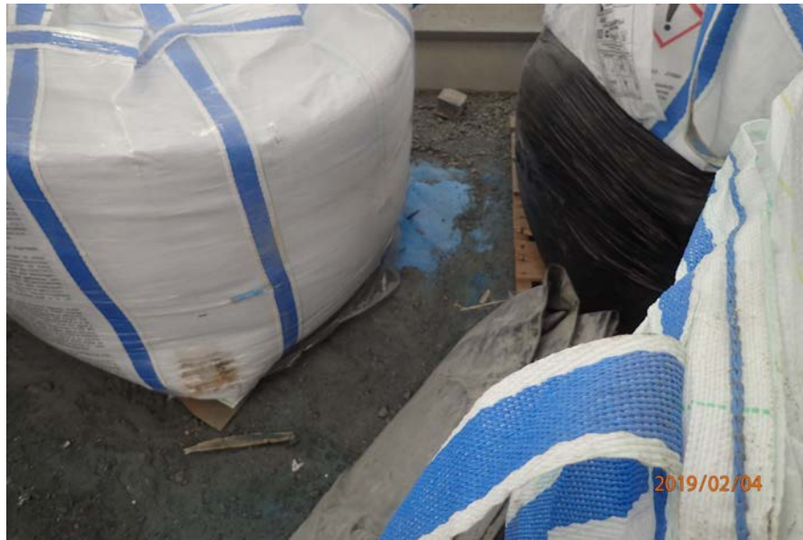
Figure 1: Example of additional damaged totes and spilled copper sulfate discovered during initial clean up.
