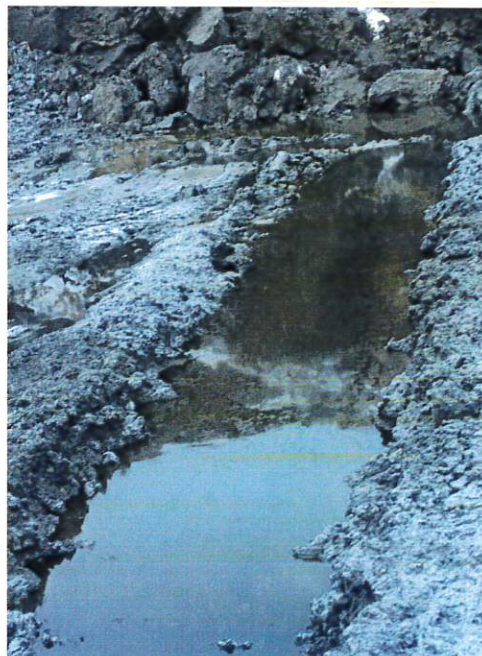
Photo 3. Hydraulic fluid collected in a berm area on floor of 300 bench.
