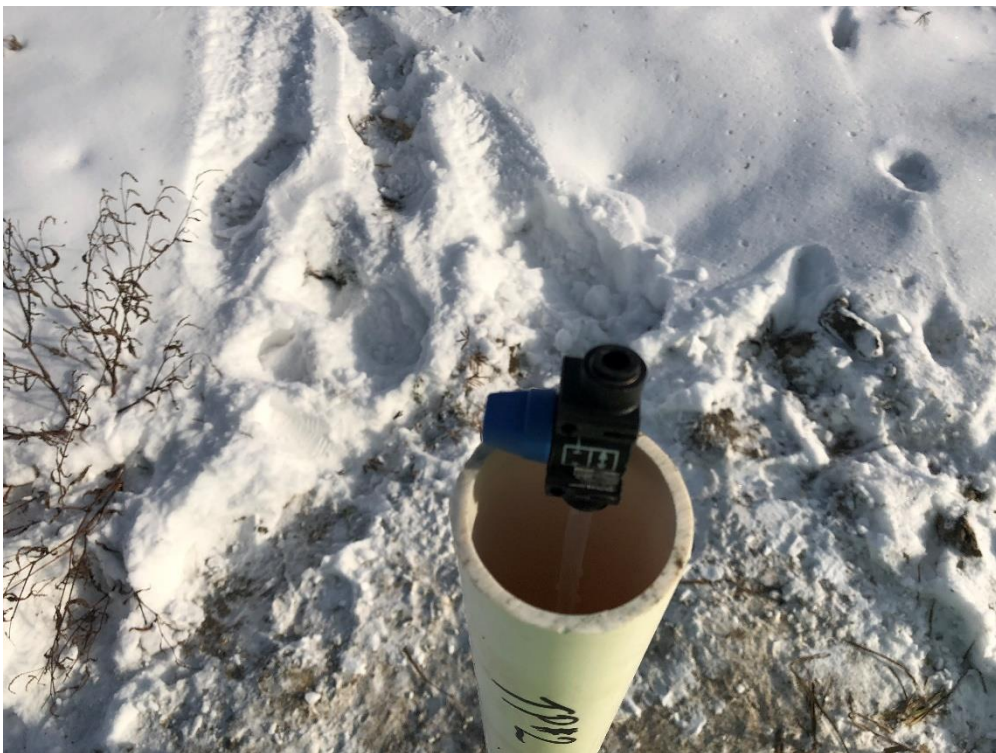
Photograph A.2: Manual gas sampling shut-off valve. November 14, 2018.
