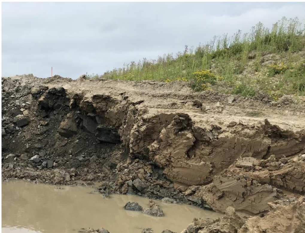
Figure 2.2: Borrow investigation of clay key layer on southeast corner of Trial #2. July 15, 2019.
