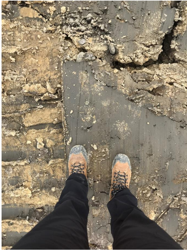
Figure 8: Slickensides indicative of a high clay content material as placed on the plateau surface.
