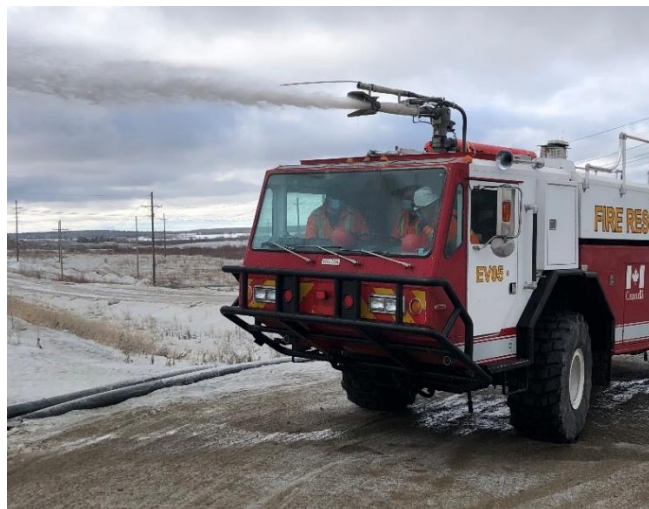
Figure 5. New Fire truck testing water canon
