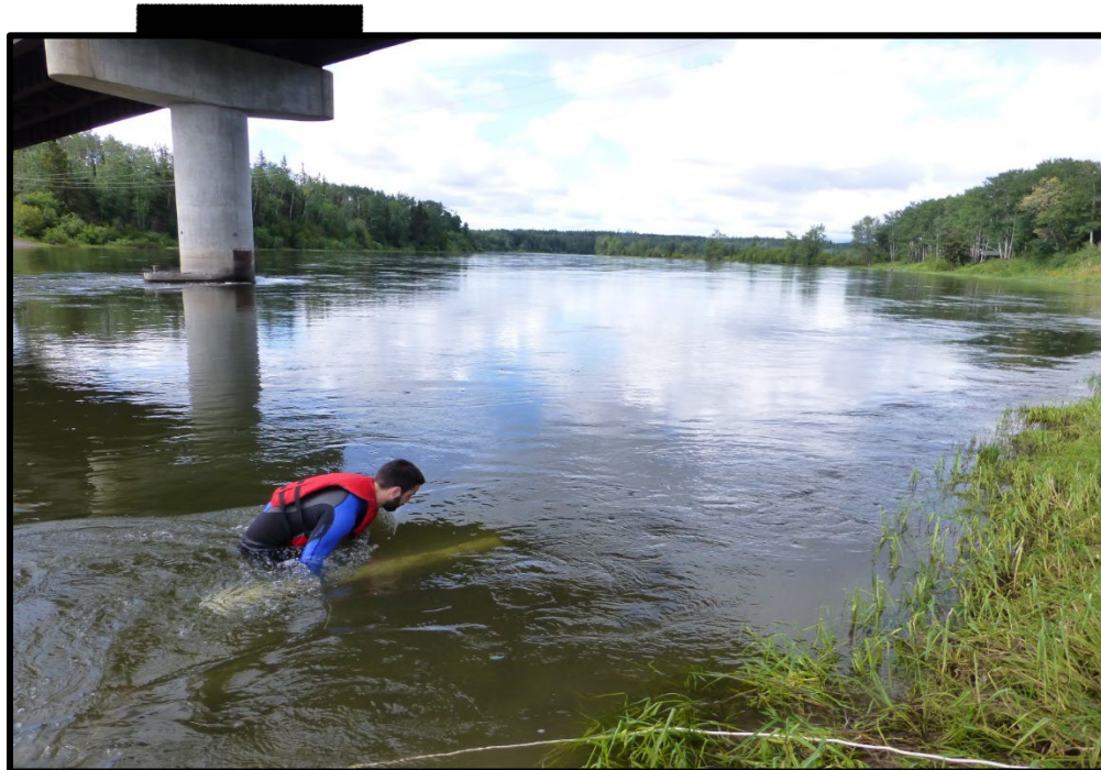
Photograph 2. Installing a sediment sampler in the Nechako River (Photo: Phil Owens).
