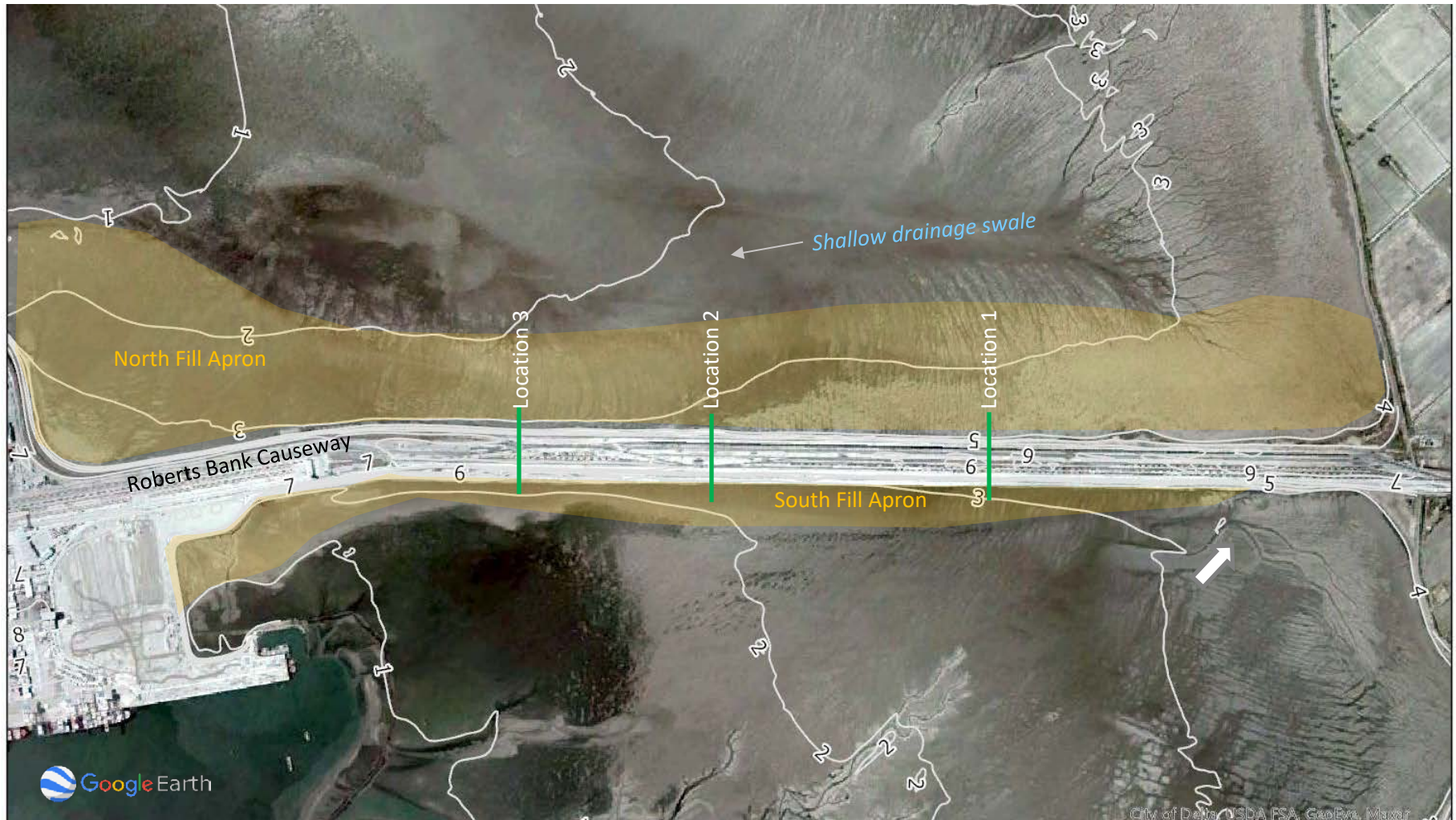
Figure 4.1 Major tidal flat features of relevance to potential channel formation at potential causeway breach locations (Google Earth imagery date April 2009). Arrow on south side of causeway indicates location of an existing channel network.
