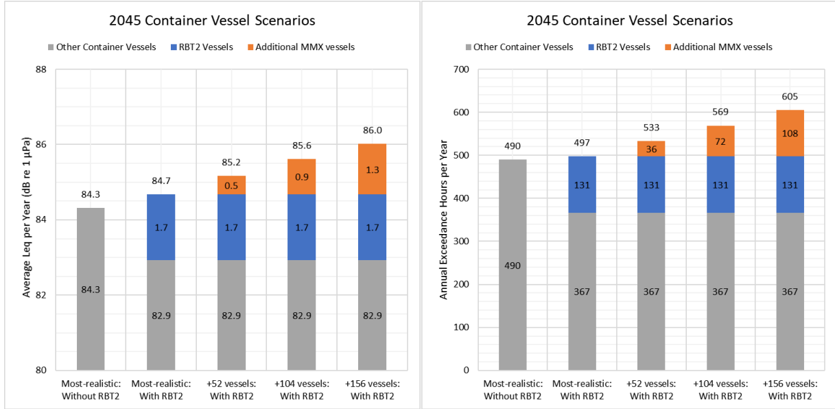
Figure B-8. 20 kHz echolocation click masking band: Average L_{eq} per year (left) and average exceedance hours per year above 20 kHz echolocation click masking threshold (right) under the most-realistic and high-case scenarios for 2045. Colors and annotations within the bars indicate the contributions of different categories of vessels (see main text for details). Annotations above the bars indicate total values. Values are averaged over Georgia Strait, Haro Strait, and Juan de Fuca Strait sub-areas. Exceedance numbers shown in the figure have been rounded to the nearest whole hour.
