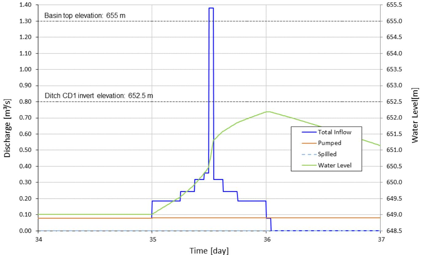
**Figure 7-1: 25 Years Flood Routing through the Transfer Basin**
