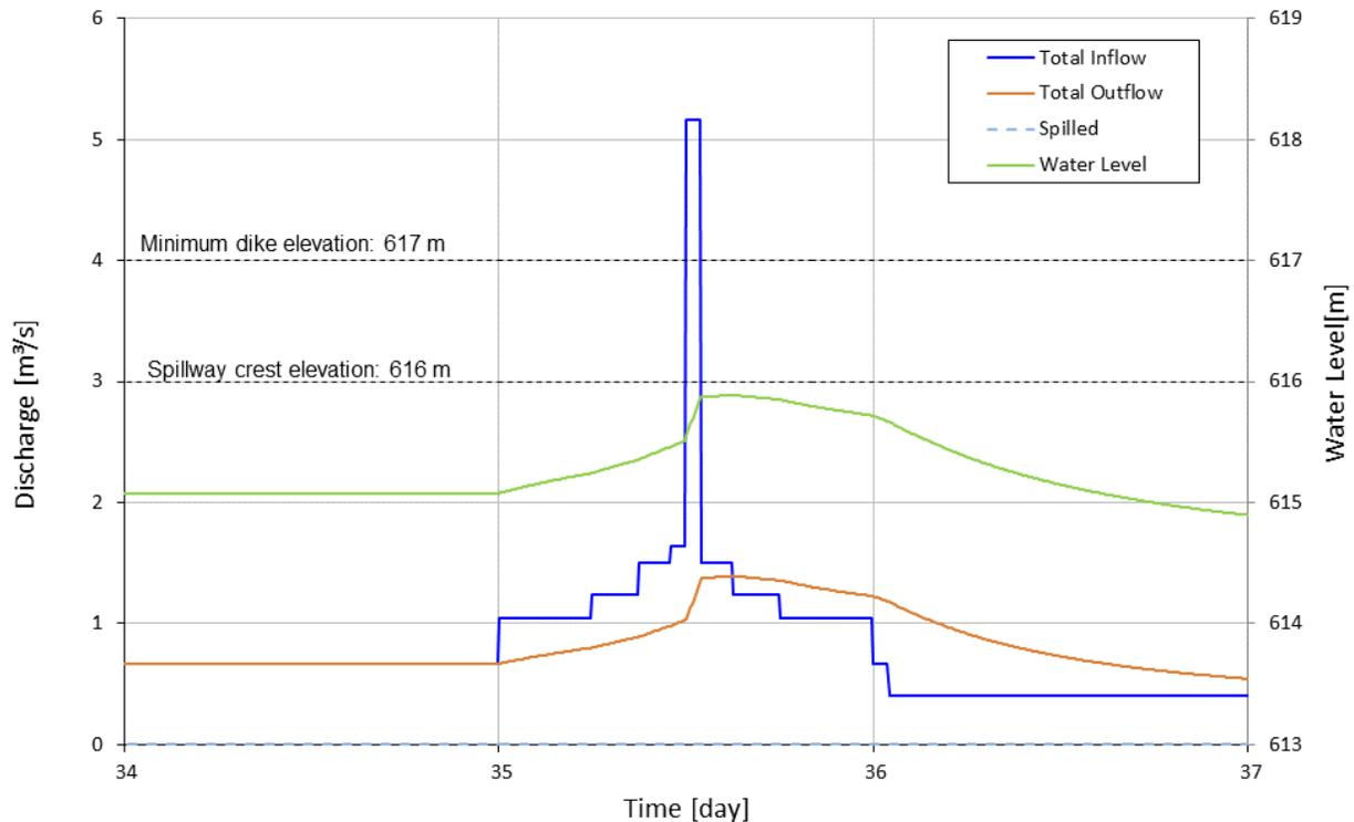
Figure 7-5: 25 Years Flood Routing through Sedimentation Pond H2
