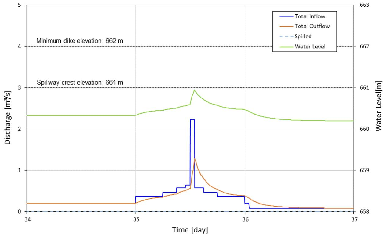
**Figure 7-3: 25 Years Flood Routing through Timmins 4 Sedimentation Pond 3**
