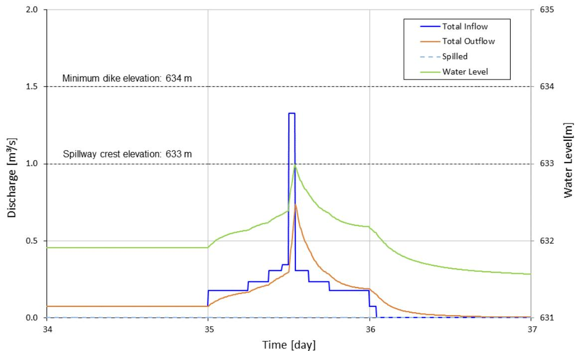
**Figure 7-4: 25 Years Flood Routing through Sedimentation Pond H1**
