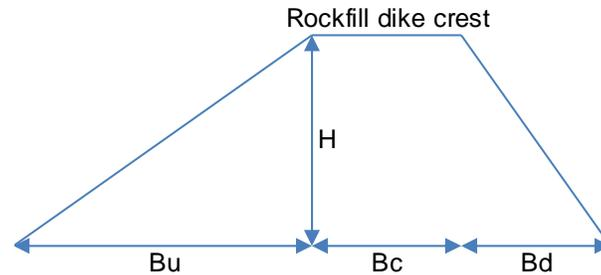
**Figure 7-2: Rockfill Dike Cross-Section Sketch**
