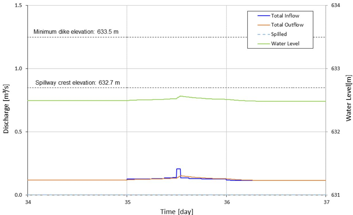
**Figure 7-6: 25 Years Flood Routing through Sedimentation Pond H3**
