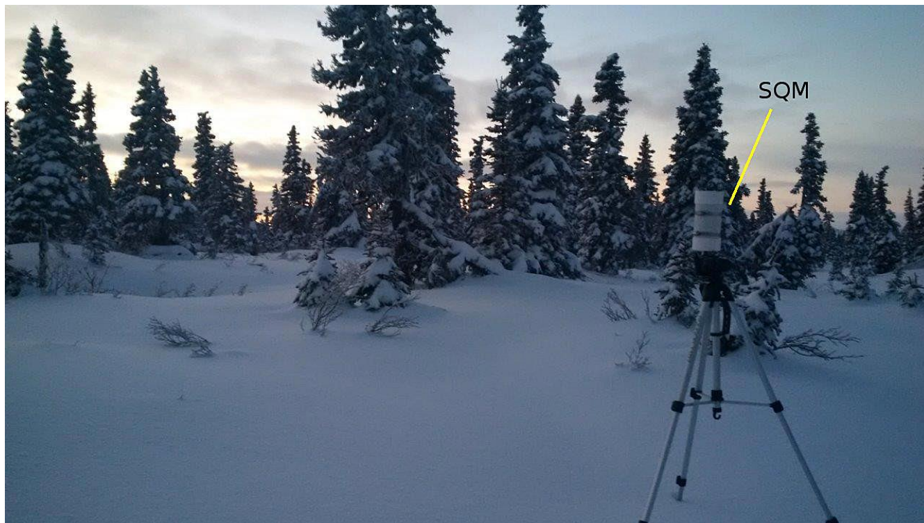
Figure 1 SQM-LU-DL with a protective housing mounted on a tripod. Credits: Denis Lalonde. AECOM
