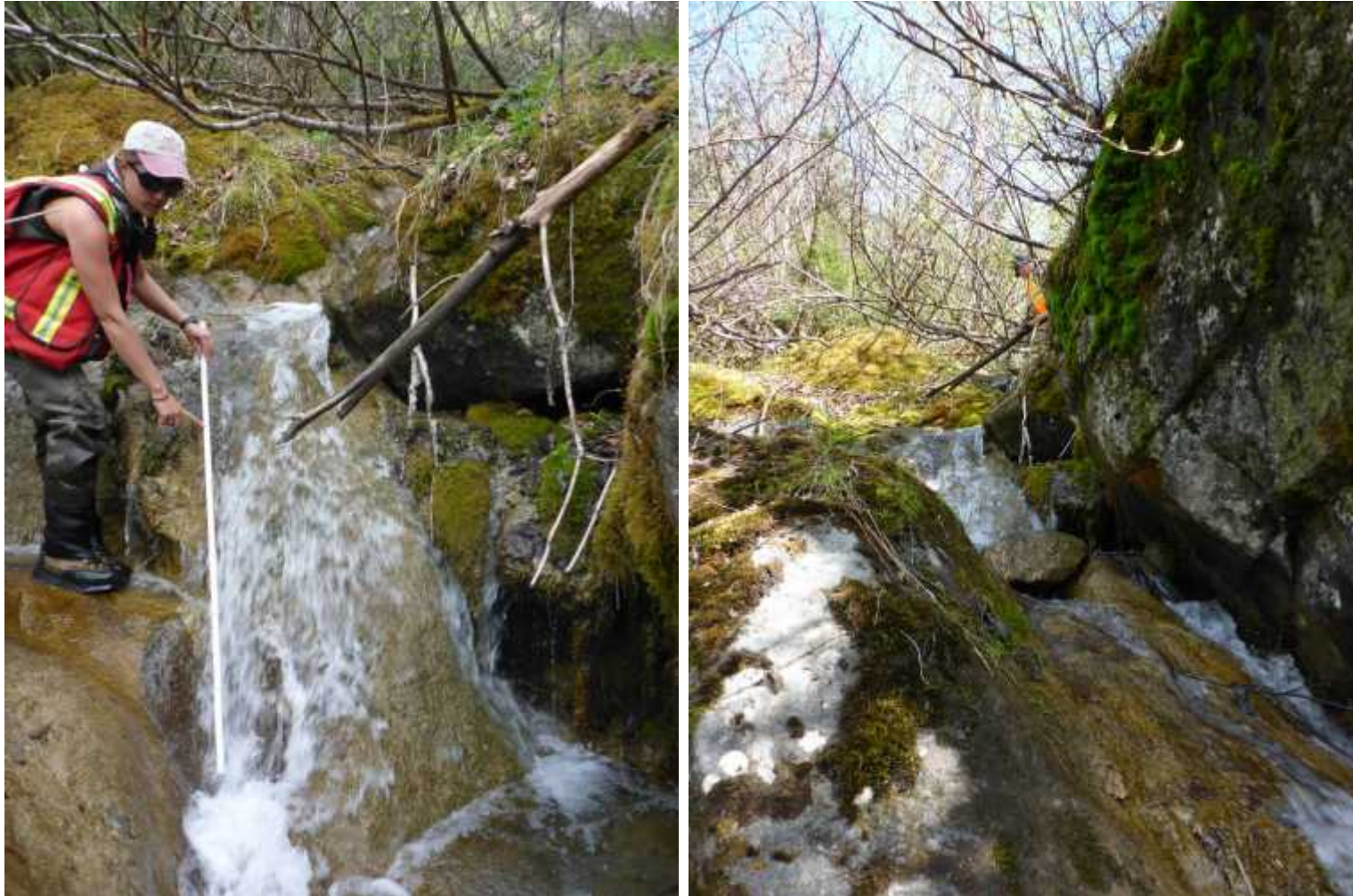
Figure 7: Chute on unnamed tributary, crew member's left index finger shows the 1 metre mark on the meter stick. Gradient was 46%. Date taken: 16-May-2017.
