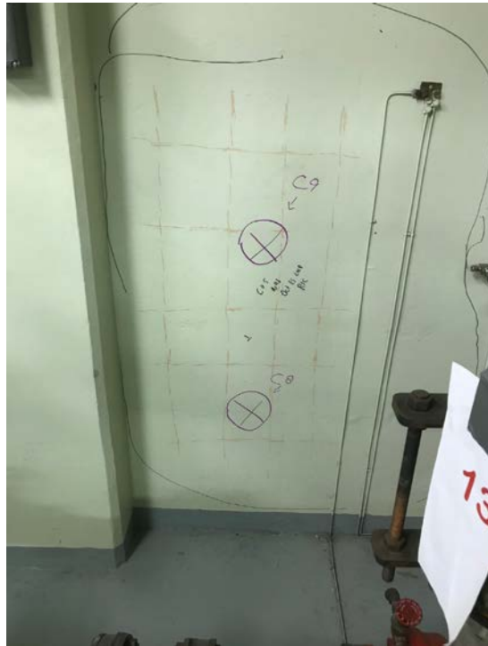
Location of Cores C8 and 9 after GPR scanning
