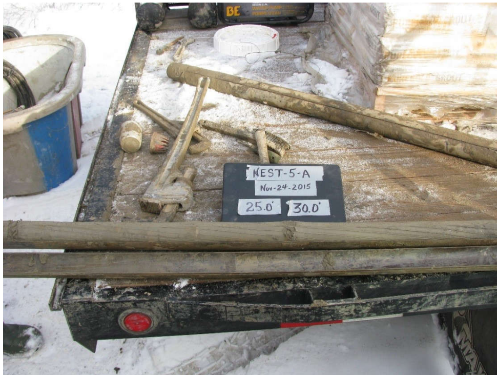
Figure 4-4: Example of Clay Core from Glaciolacustrine Clay Deposit Near WR-1
