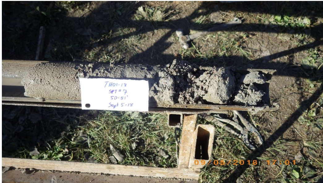
Figure 4-7: Example of Basal Till Core near South End of Main Campus. Note larger grained-sized particles would not be able to be captured in the core barrel.
