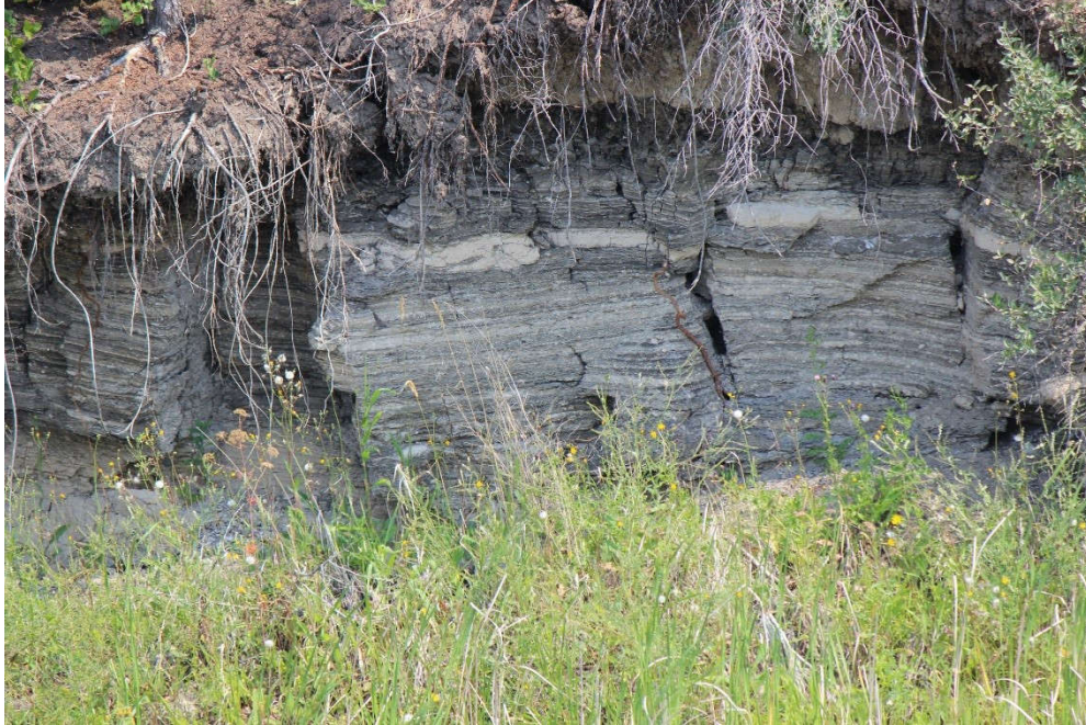
Figure 4-1: Example of the Varved Nature of the Glaciolacustrine Clay. Erosional exposure along the Winnipeg River near the WL Site, fissuring due to slumping of the clay (Collection of the Author).
