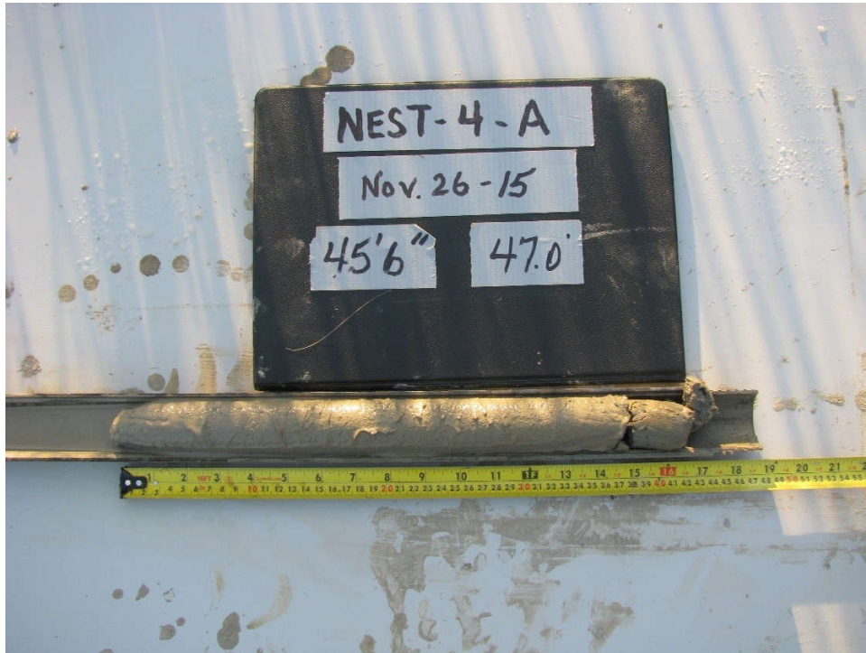
Figure 4-5: Example of Clay Till Core Near WR-1
