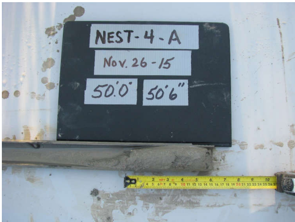
Figure 4-6: Example of Basal Till Core Near WR-1. Note larger grain-sized particles would not be able to be captured in the core barrel.
