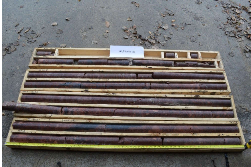
Figure 4-11: Rock Core from Shallow Bedrock Borehole 16-8A. Rock shows reddish alteration and dipping fractures.
