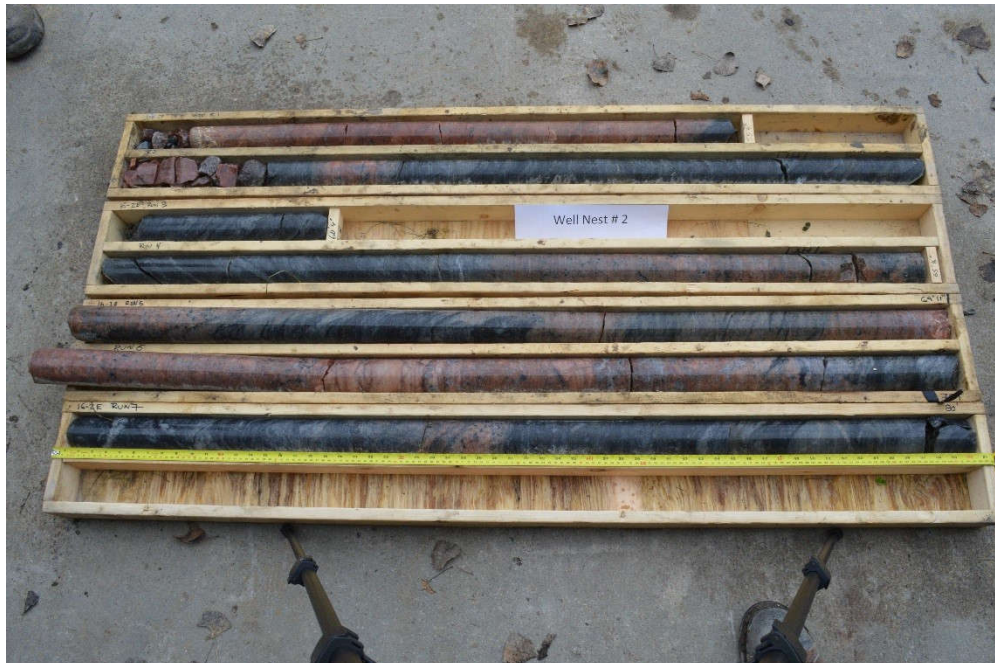
Figure 4-8: Rock Core from Shallow Bedrock Borehole 16-2E. Broken core sections indicate areas of fractured rock, mafic banding, which may be related to a mafic dyke or xenolithic structure, are present.
