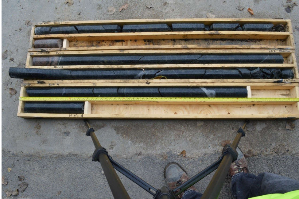
Figure 4-9: Rock Core from Shallow Bedrock Borehole 16-4F. Mafic rock, likely due to the presence of a mafic dyke, is present.
