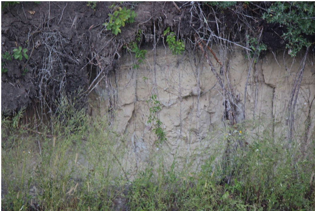
Figure 4-2: Example of Weathered Clay Till Erosional Exposure along the Winnipeg River near the WL Site. Some gravel-sized grains are visible (Collection of the Author).
