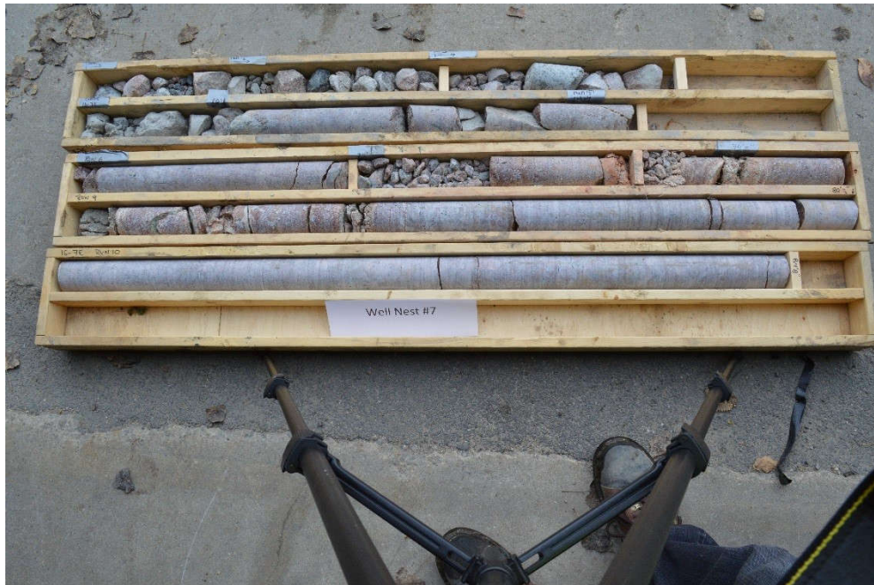
Figure 4-10: Rock Core from Shallow Bedrock Borehole 16-7E. Zones of Rubblized core indicating fractured rock is present.
