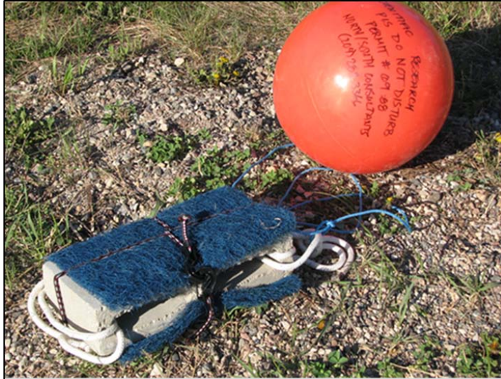
Figure 7-3. An egg mat ready for deployment.
