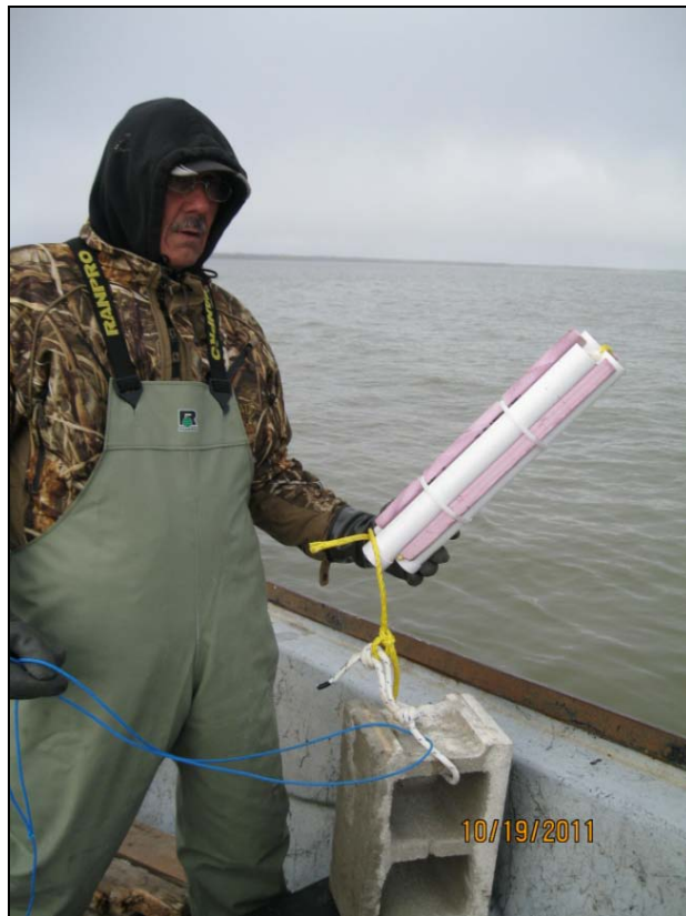
Figure 4-3. Example of sediment trap deployed in Sturgeon Bay.
