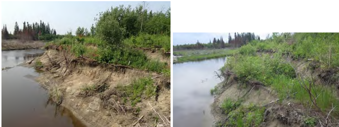
25+000: Bank slump on left side of creek, looking upstream in 2013 (left) and 2014 (right).
