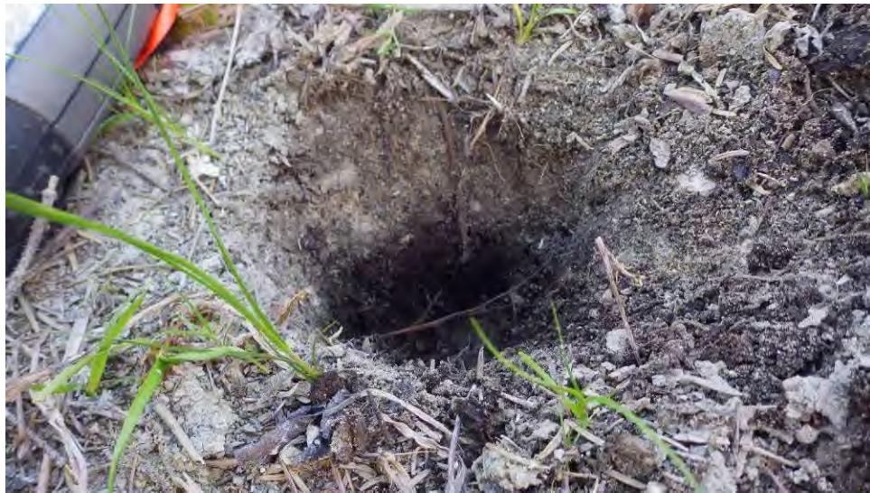
Photo 12. Soil sampling hole at 19+500 showing organic soils (black) overlain by inorganic soils (grey).
