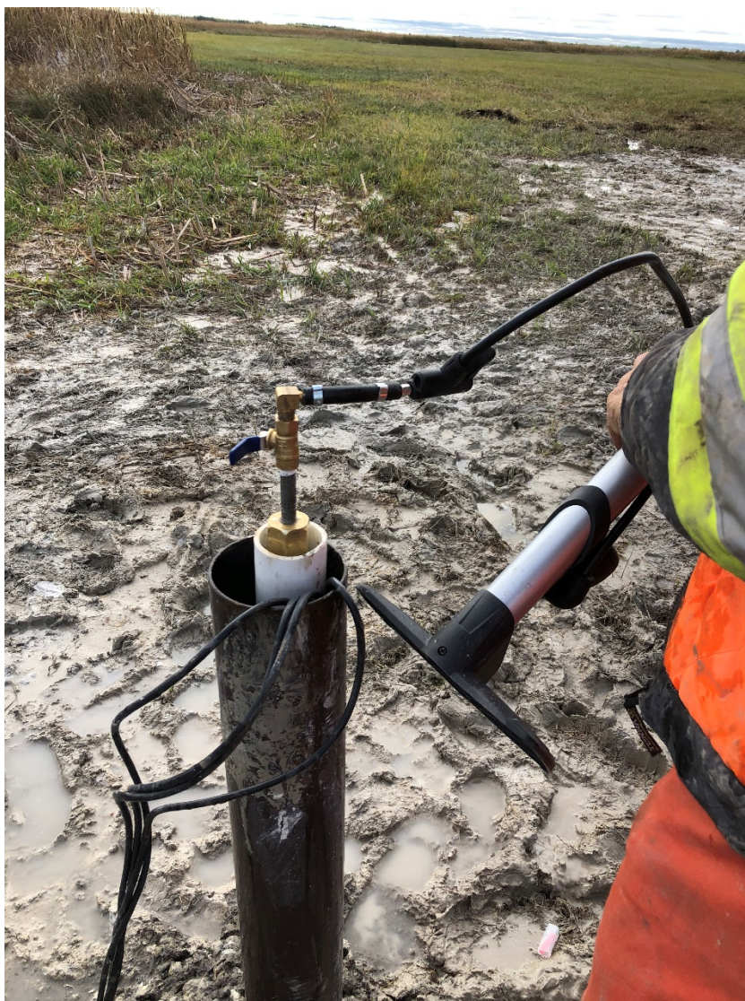
Figure 3-1 Groundwater Well Preparation for Winter Months including Packer Installation
