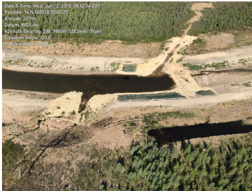
Figure 3 – June 2019 aerial view of the Creek 3 plug, looking west. The leaky flow through this plug (to the right or dry side of the plug), proceeds down channel into the bedrock exposed area of Reach 3 of the EOC. The metered flow contribution calculated at the down channel bedrock exposed area of Reach 3 was 0.004 M 3 /s at this time.
