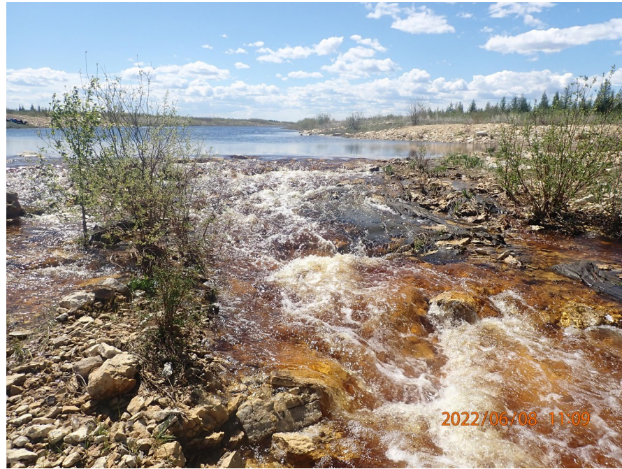
Figure 1 – June 2022 view of the Creek 3 plug, looking up channel. The flow over this plug proceeds down channel into the bedrock exposed area of Reach 3 of the EOC. The metered flow contribution calculated at the down channel bedrock exposed area of Reach 3 was 0.18 M 3 /s at this time.
