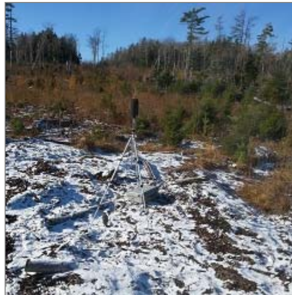
Photo 2: Sound Meter System 824
