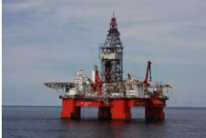
Figure 2.3 Typical Offshore Drilling Units: Semisubmersible Drilling Unit
