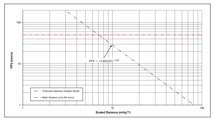
Figure 2: Ground Vibration Attenuation Models for the Valentine Project Open Pits.
