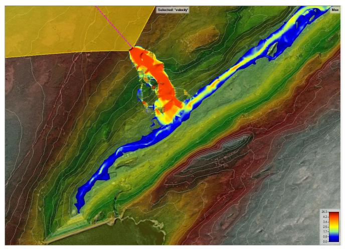
Figure 32: Processed Results showing Maximum Velocities (m/s) Immediately Downstream the TMF –South Dam Breach Failure (Scenario C)
