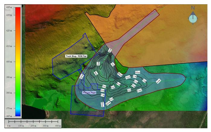
Figure 34: Tailings Runout Deposition for the TMF West Dam Failure (Scenario D) with Process Plant Inundated
