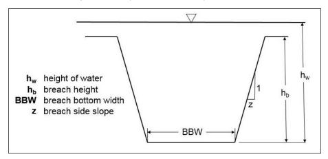
Schematic 1: Parameters of an Idealized Dam Breach
