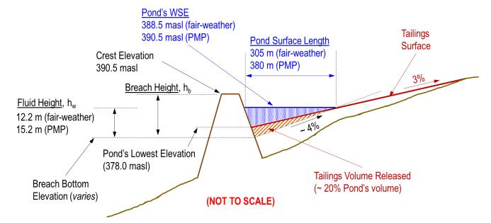
Schematic 2: Conceptual Breach Channel Profile
