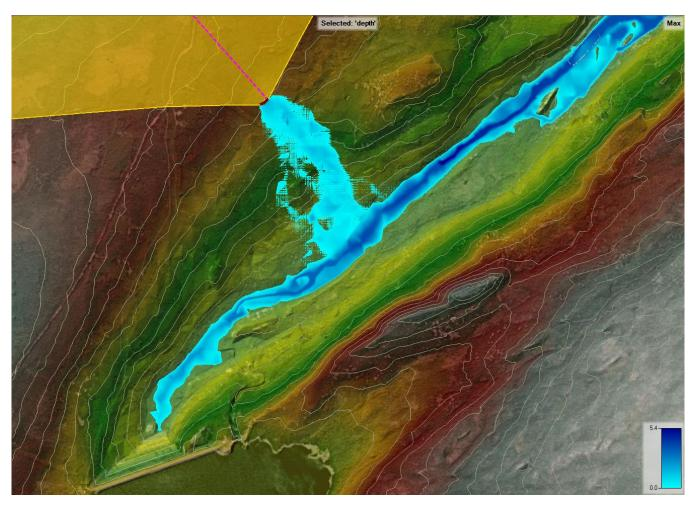
Figure 33: Processed Results showing Maximum Water Depths (m) Immediately Downstream the TMF – South Dam Breach Failure (Scenario C)
