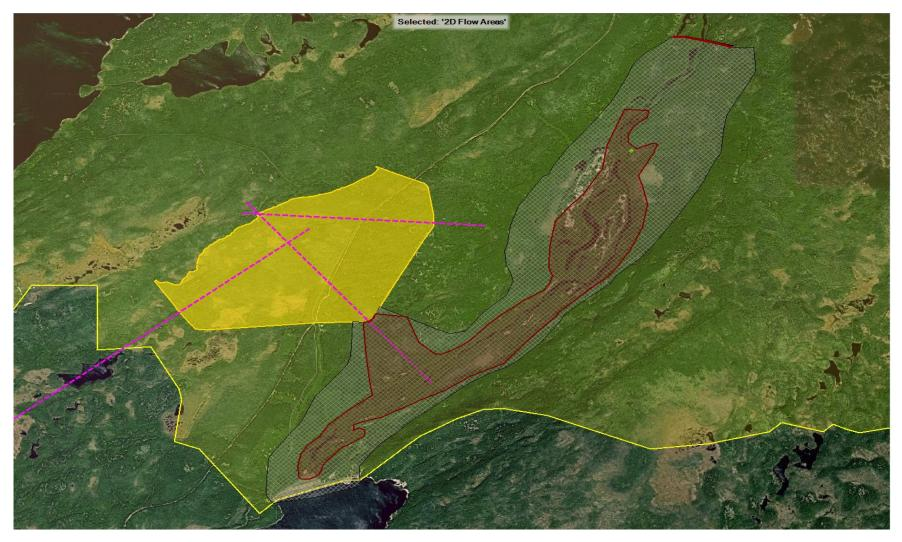
Figure 14: Hydrologic and Hydraulic Model Boundary for the TMF South Dam Failure Simulations (Scenario C)
