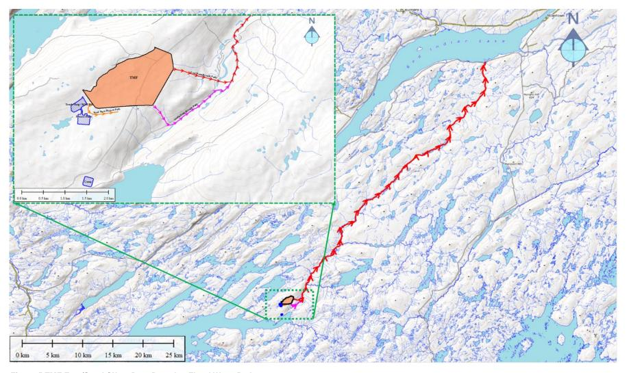
Figure 5 TMF East/South/West Dam Breach – Flood Wave Paths
