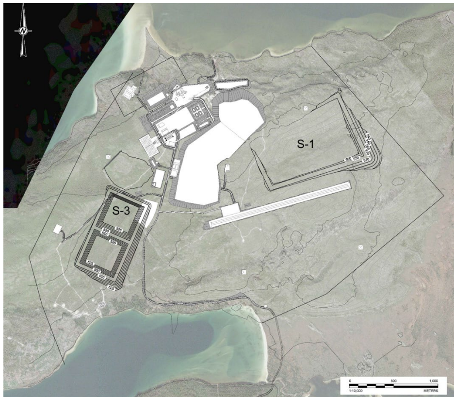
Figure 13: Conceptual Plan Illustration of the Surface Paste Technology Alternatives at Locations S-1 and S-3
