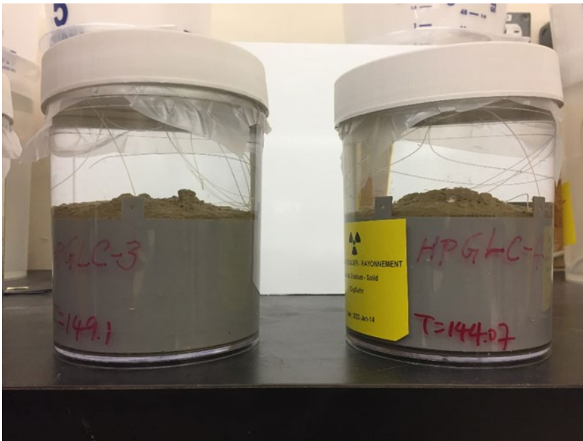
Figure 5-2: Leaching Environmental Assessment Framework Compacted Granular (1-Dimensional) Sample Swelling
