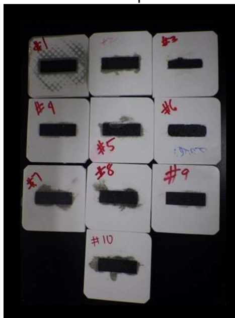
Figure 7. Fine (<1mm) Troilus J4 rock samples mounted on epoxy and polished for XRD analysis.
