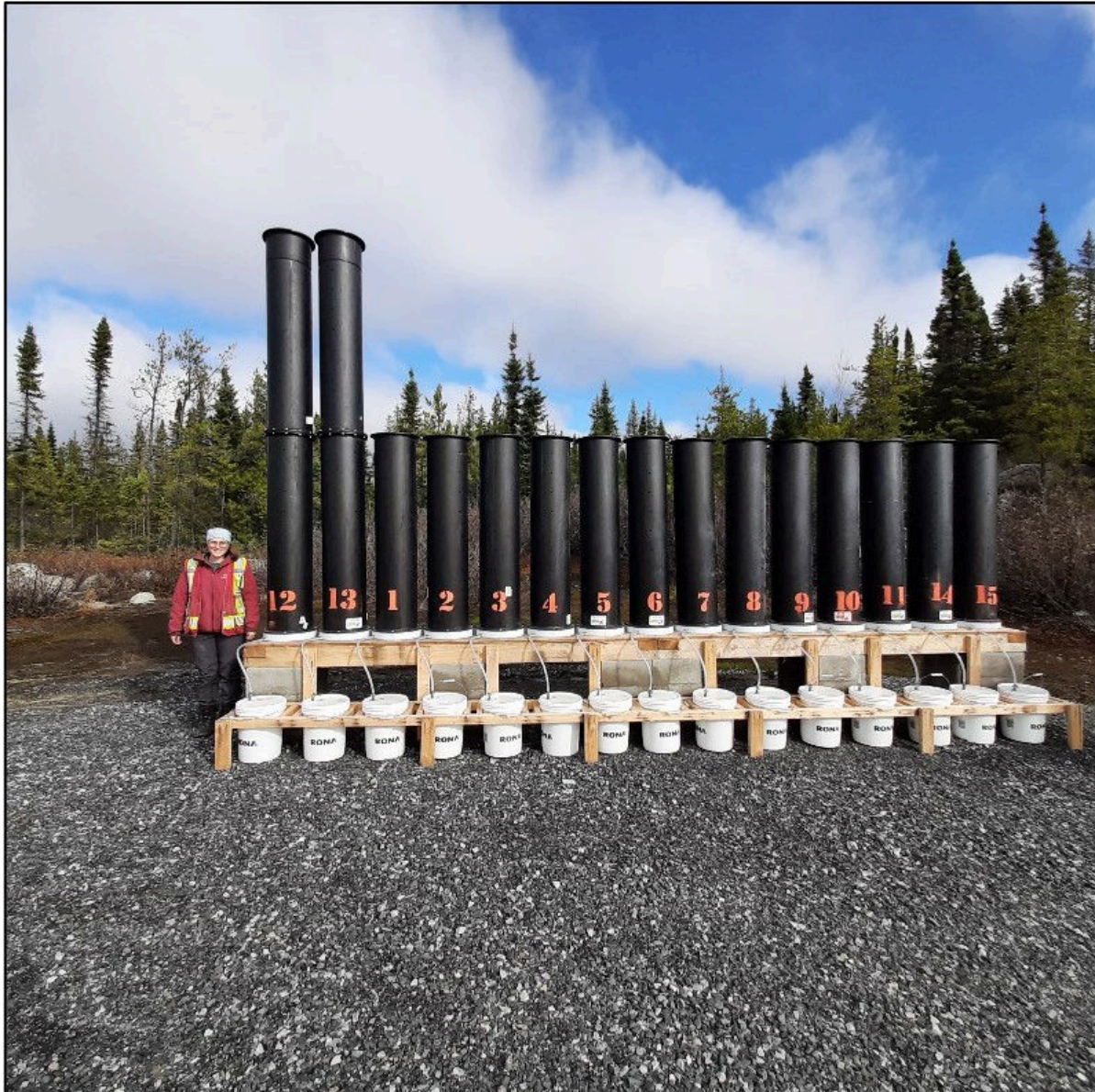
Figure 3-2. A photograph of the 13 on-site ML-ARD columns, with Columns 12 and 13 containing hundreds of kg of existing, weathered J4 waste rock.
