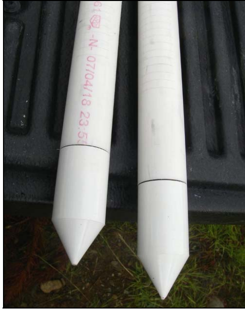
a) Well materials. These consisted of 152 cm long, 2.5 cm diameter, slotted PVC piping with a drive point end. Photo taken: June 2008.
