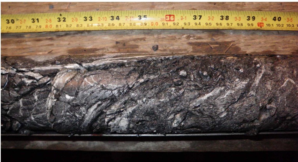
Photo 2.23 KC09-10 15.5 m Clay Gouge Layers in Weathered Fault Zone within Metasediments.
