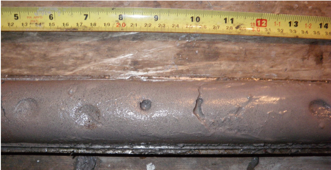
Photo 2.19 KC09-09 2.5m thick layer of Silty Fine Sand at 73 m.
