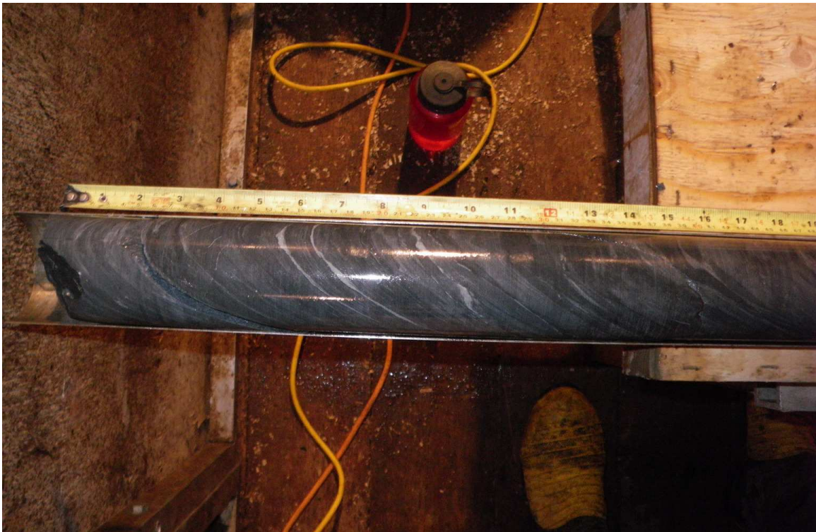
Photo 2.26 Typical Core from KC09-13, bedded argillite with quartz veins (10.5 m to 11.0 m).
