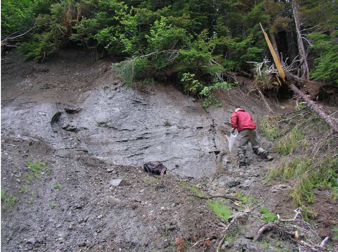
Photo 2.12 Dense, consolidated silty to clayey High Plasticity Lacustrine Deposit, Situated beneath Moraine Deposits, Valley Bottom at Mitchell-McTagg Confluence. Sample Site 37.
