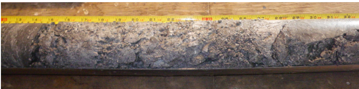
Photo 2.17 KC09-08 Fault Zone Consistent with Location of Sulphurets Thrust Trace. Depth 44 m.
