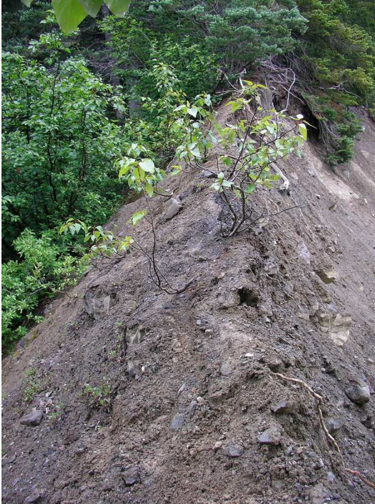
Photo 2.11 Eroded knife edge of 30 m high silty to sandy gravel. This is a moraine deposit situated over basal till and lacustrine silt layers at confluence of McTagg and Mitchell creeks.
