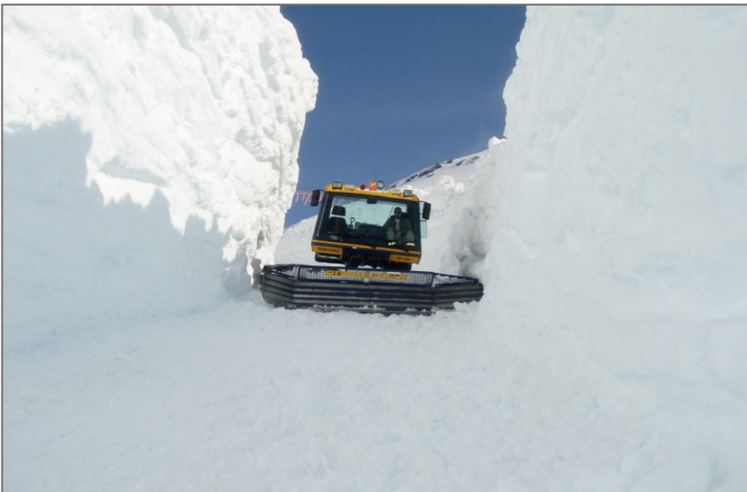
Photo 12: Photo from Brett Wildman of Nuna taken in the winter of 2009 showing a snowcat creating access trails in the area immediately south of the Eskay Creek Mine.
