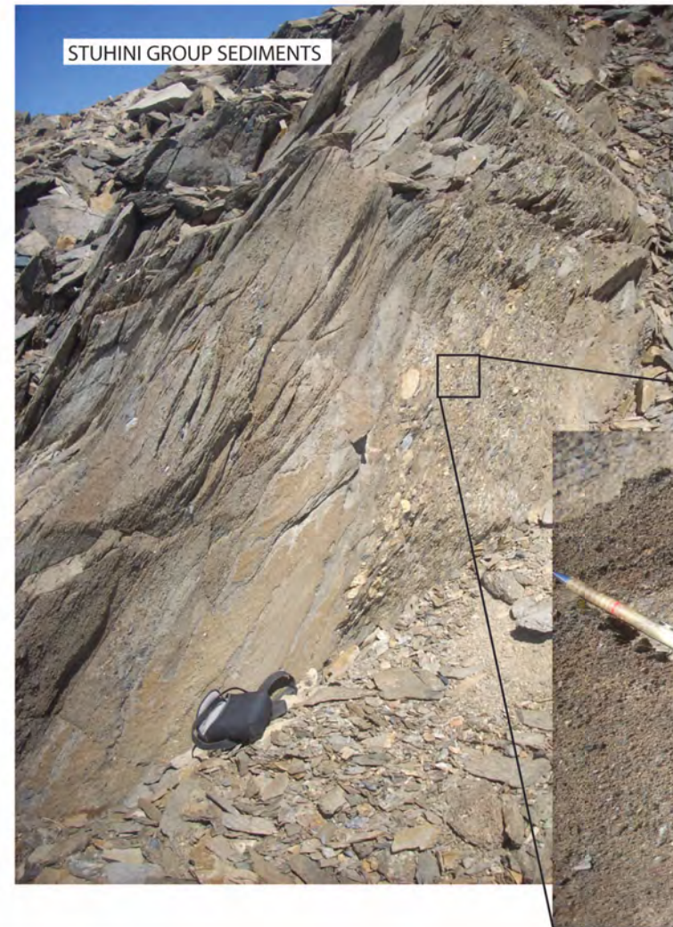
Volcanoclastics / Breccia with phyllite beds. Blue-black; to brown R3-R4; clastis 5cm diameter; matrix supported; clastis show some alignment parallel to foliation. Local qtz veinlets. GSI=45-55.
