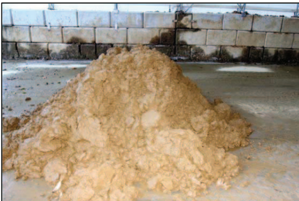
Truck Dump Load of Sludge
