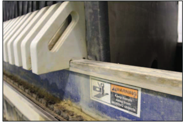
Close-up Filter Press Plate Hangers
