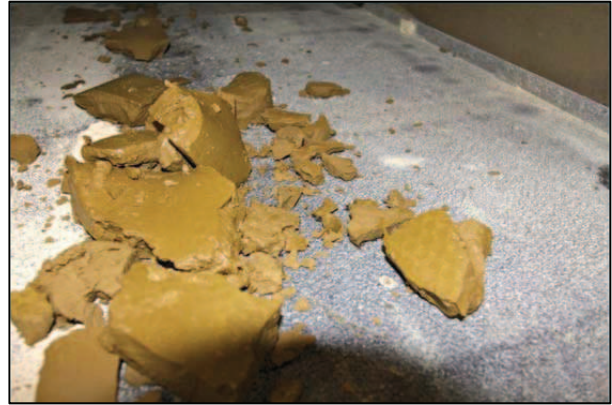
Sludge Filter Cake: 40% Moisture
