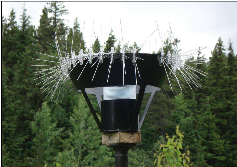
Plate 2.3-2. Close up view of a dustfall collector and wind screen. Bird spikes surround the wind screen and prevent contamination of the samples from birds.
