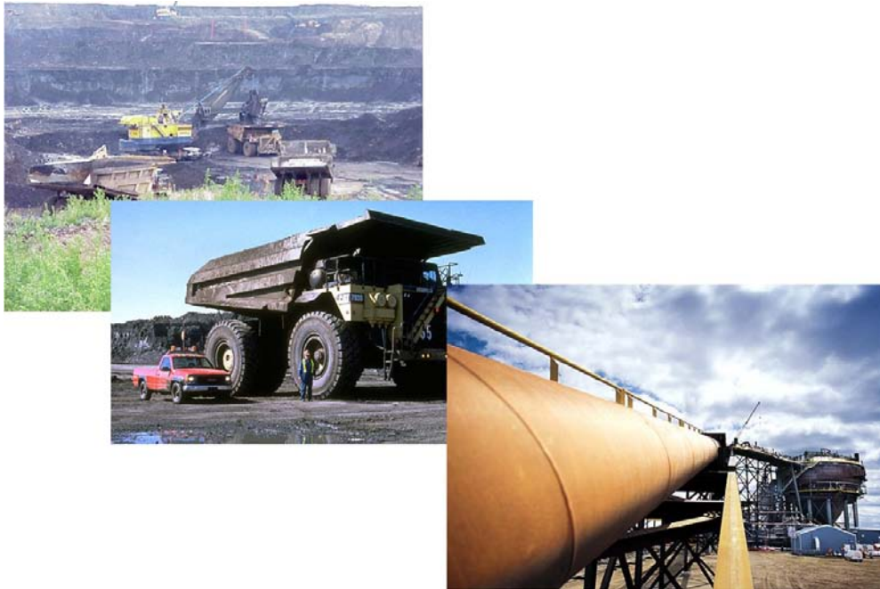
Figure 4.7 Transport of large quantity of oil sands ores by large trucks contributes to the energy intensity of bitumen production from oil sands
