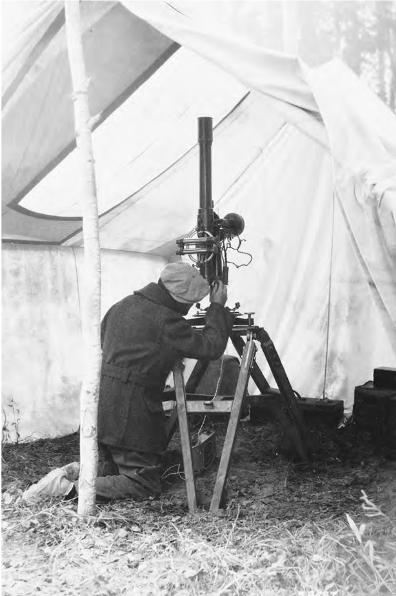
PHOTO 5.10 Zenith telescope set up for observing the northern boundary of Alberta, 1924. | Library and Archives Canada, Dept. of Mines and Technical Surveys, PA-019667
